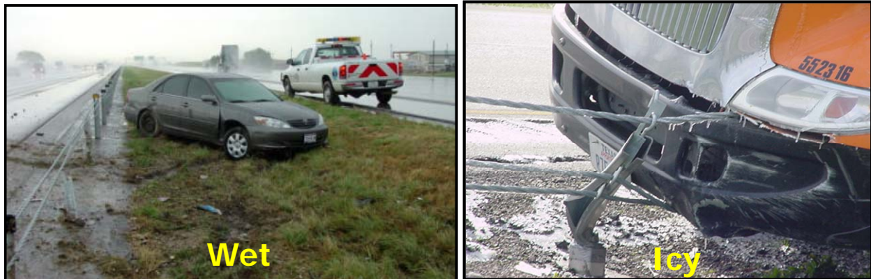
Figure 5-5. Weather Conditions Have a Significant Impact on Cable Barrier Impacts.
