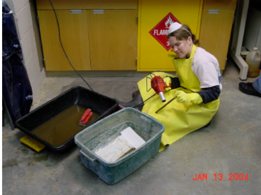
Figure 3.33 – Drying the Bars After the Chemical Bath
