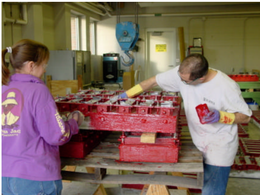
Figure 3.14 - Epoxy Coating of the Slabs and Specimens
