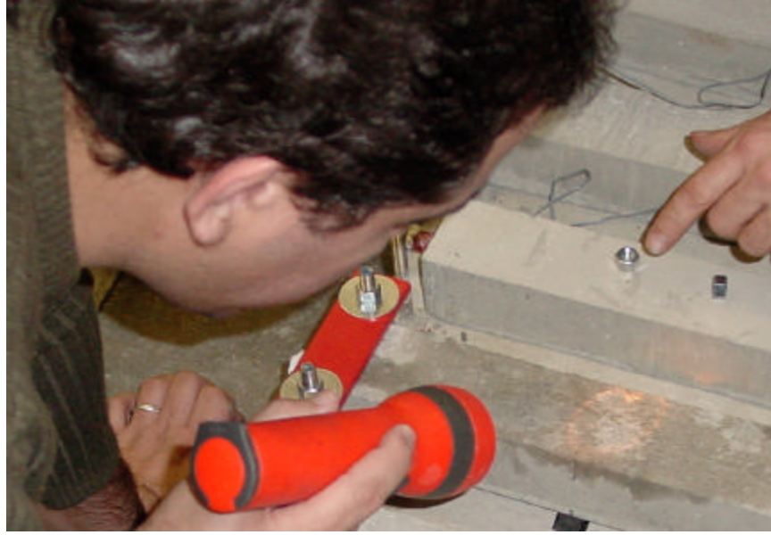
Figure 3.13 – Pilot Test 2: Spotting Cracks
