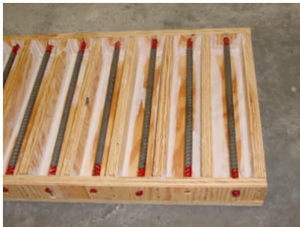
Figure 3.2 – Formwork for the Specimens
