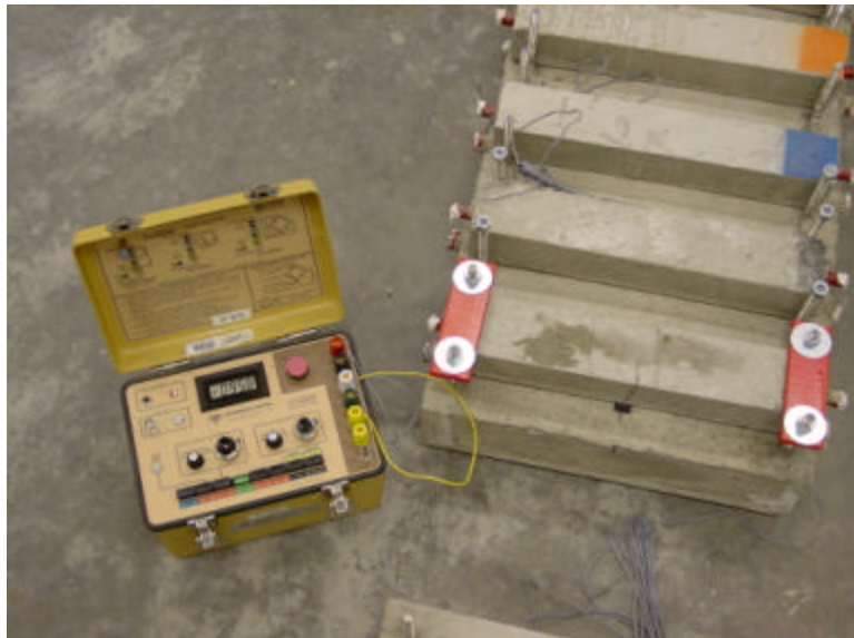
Figure 3.11 – Pilot Test 2: Setup with Strain Indicator Box
