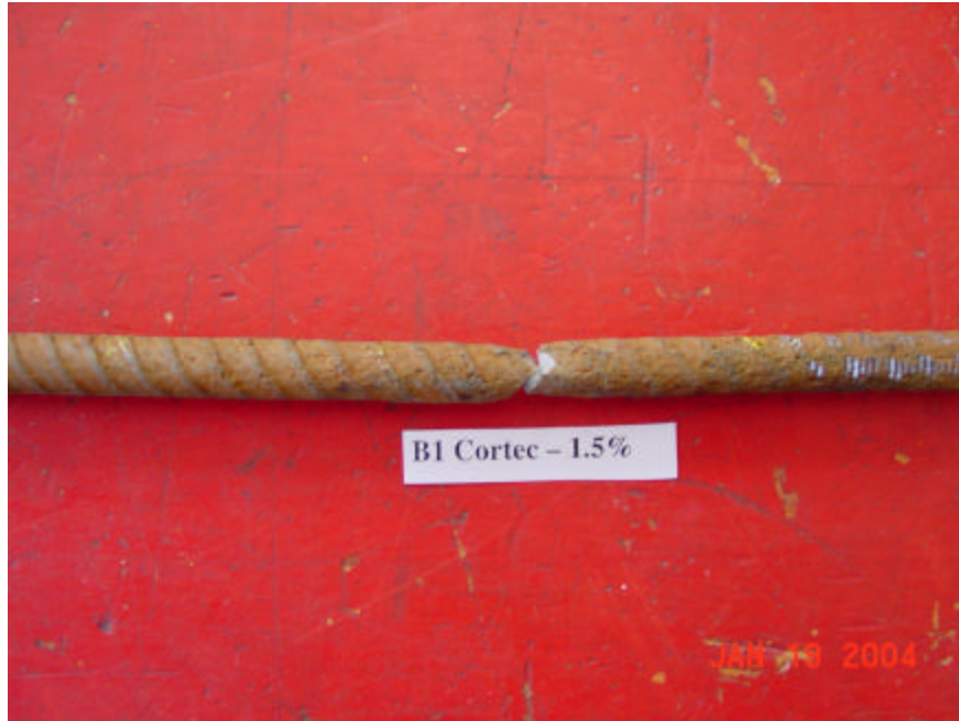
Figure 3.37 – Bar After Failure in Tension
