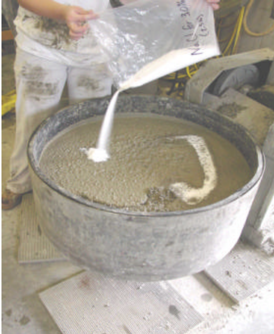
Figure 3.4 – Chloride Addition During Specimen and Cube Casting
