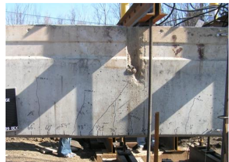
Figure 1.13 Representative flexural distress (Lake View Drive INTERIOR test girder; Harries 2006).
