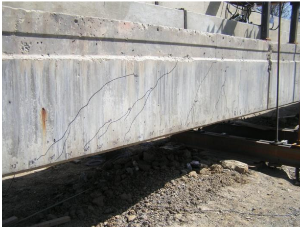
Figure 1.12 Representative shear distress (Lake View Drive EXTERIOR test girder; Harries 2006).
