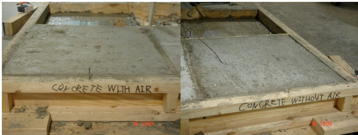
Figure 2.10. 2 ft x 2 ft NA and NN concrete placed in forms
