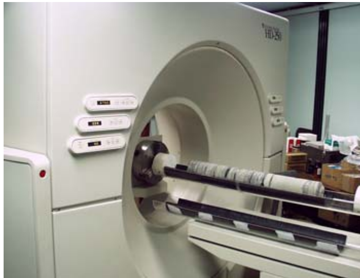
Figure 1.12. Universal HD-350 medical scanner at Penn State
