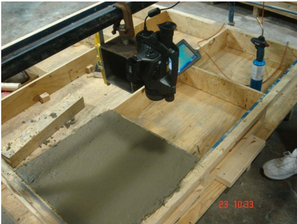
Figure 2.24. Infrared camera mounted on frame above concrete slab
