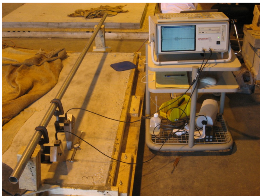
Figure 2.9. Rayleigh wave test setup on hardened concrete
