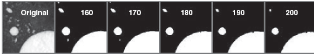
Figure 1.17. Example of threshold value comparison (Carlson, 2006)
