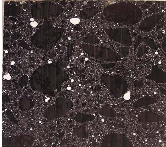
Figure 1.6. Image of specimen surface after contrast enhancement (Jakobsen et al., 2006)
