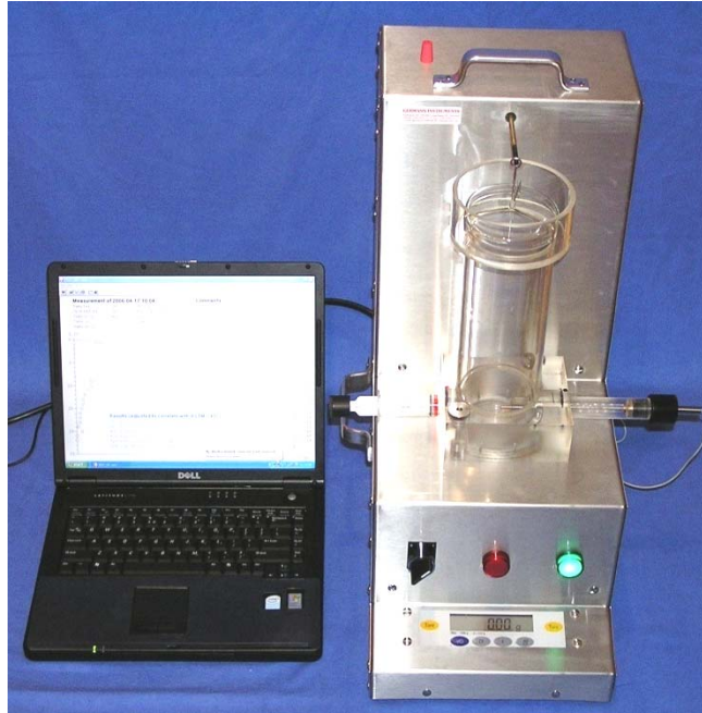
Figure 1.4. Air Void Analyzer (Germann Instruments, Inc., 2008)
