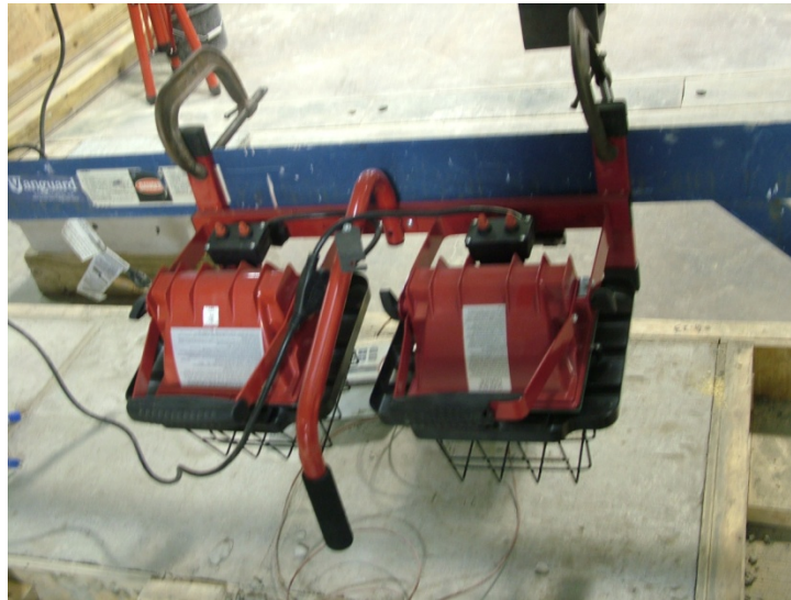
Figure 2.25. Setup for halogen lamp heating
