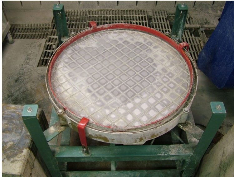
Figure 2.3. Vibro lap polishing machine
