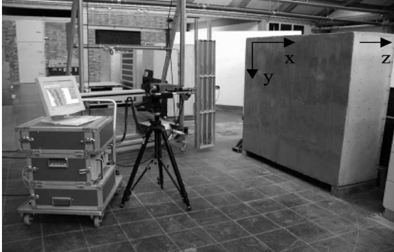
Figure 1.23. Experimental set-up for the measurement of impulse-thermography (Maihofer et al., 2003)
