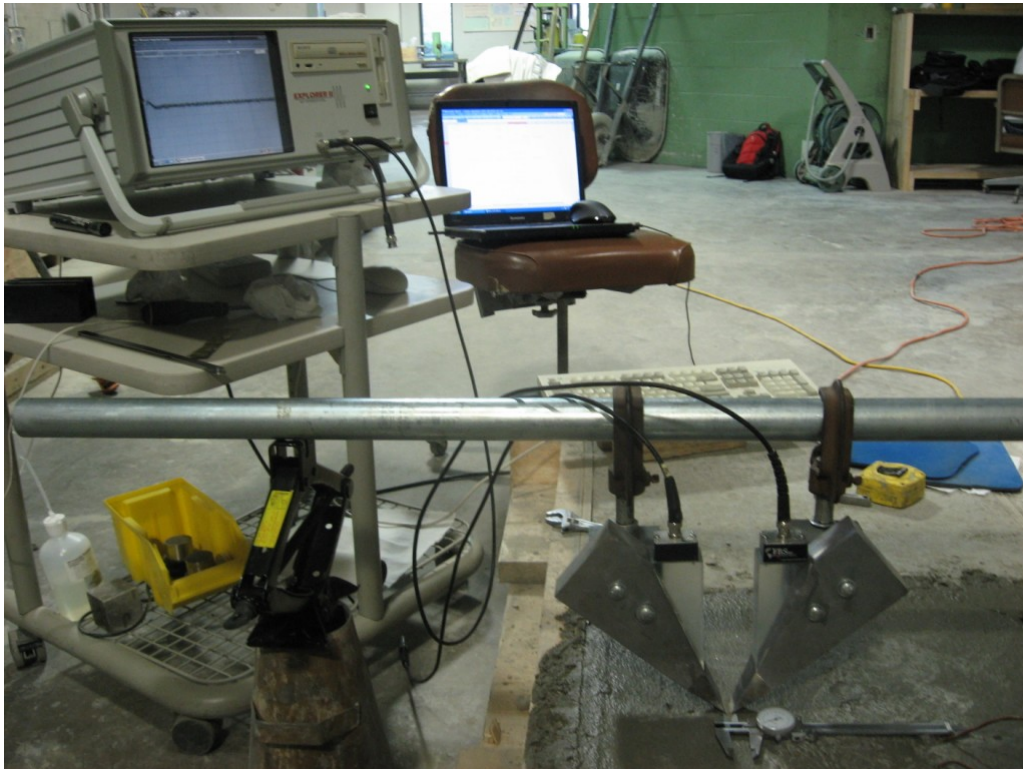
Figure 2.4. Rayleigh wave test setup on fresh concrete
