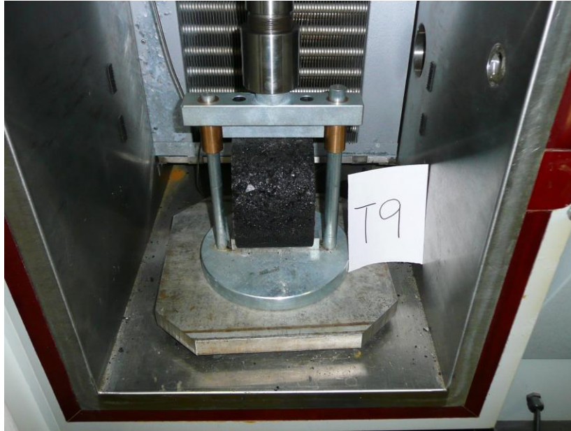
Figure 4 SGC Specimen Set in the Loading Frame for Indirect Tensile Testing
