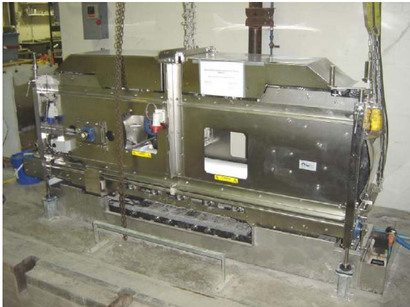
Figure 7 MMLS3 on Top of the Test Bed
