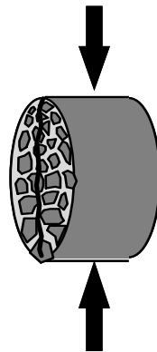
Figure 5 Testing in Diametral Direction to Determine Indirect Tensile Strength
