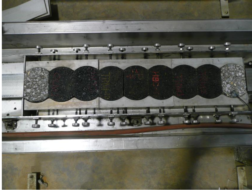
Figure 6 Briquettes are Placed in the Test Bed before Mounting MMLS3
