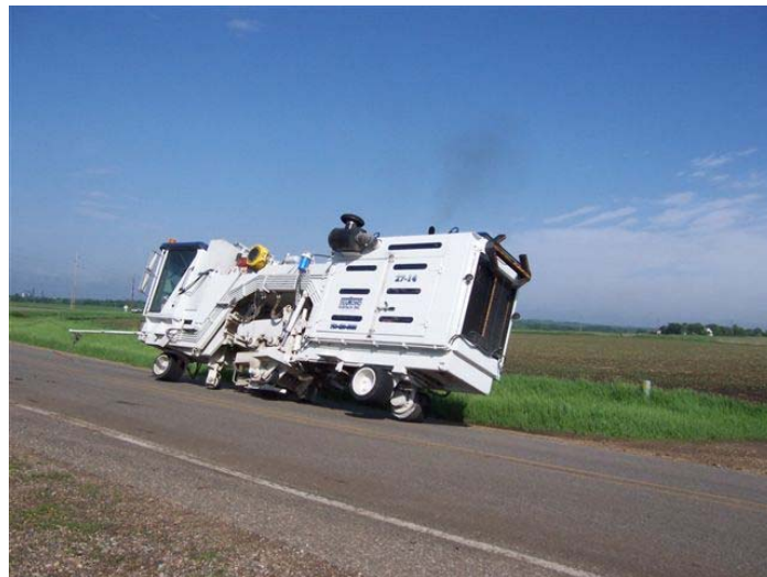
Figure 3-11. Machine tipping on inside curve
