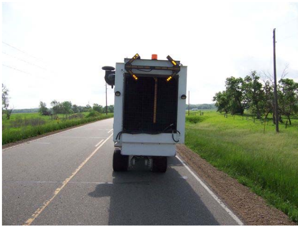
(b) Side-shift left—provided most weight over mill head
