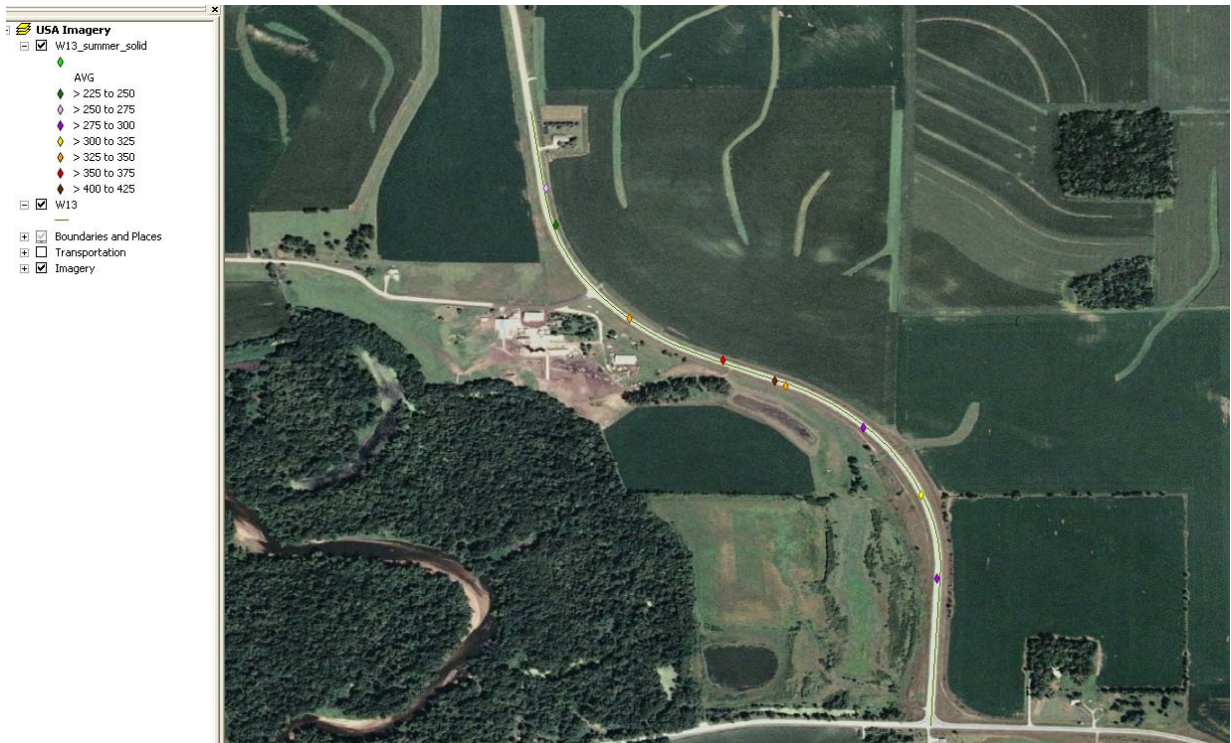
Figure 5-7. Summer readings for control for test section W-13
