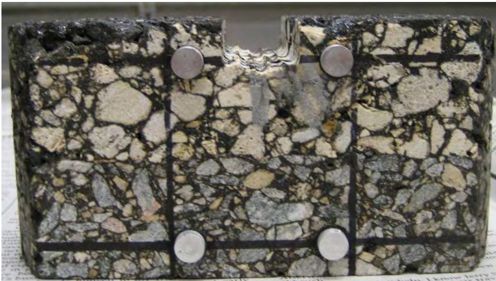
Figure 5-21 Prepared Composite Specimen with Diamond Saw Cut Groove
