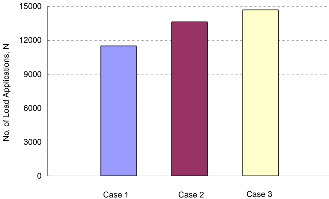
Figure 6-33 Loading Cycles to create 0.4 inch crack in the Local Model
