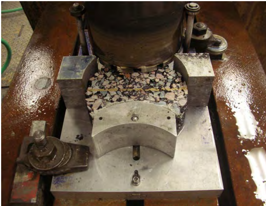
Figure 4-12 Coring the Other Side of Asphalt Mixture Sliced
