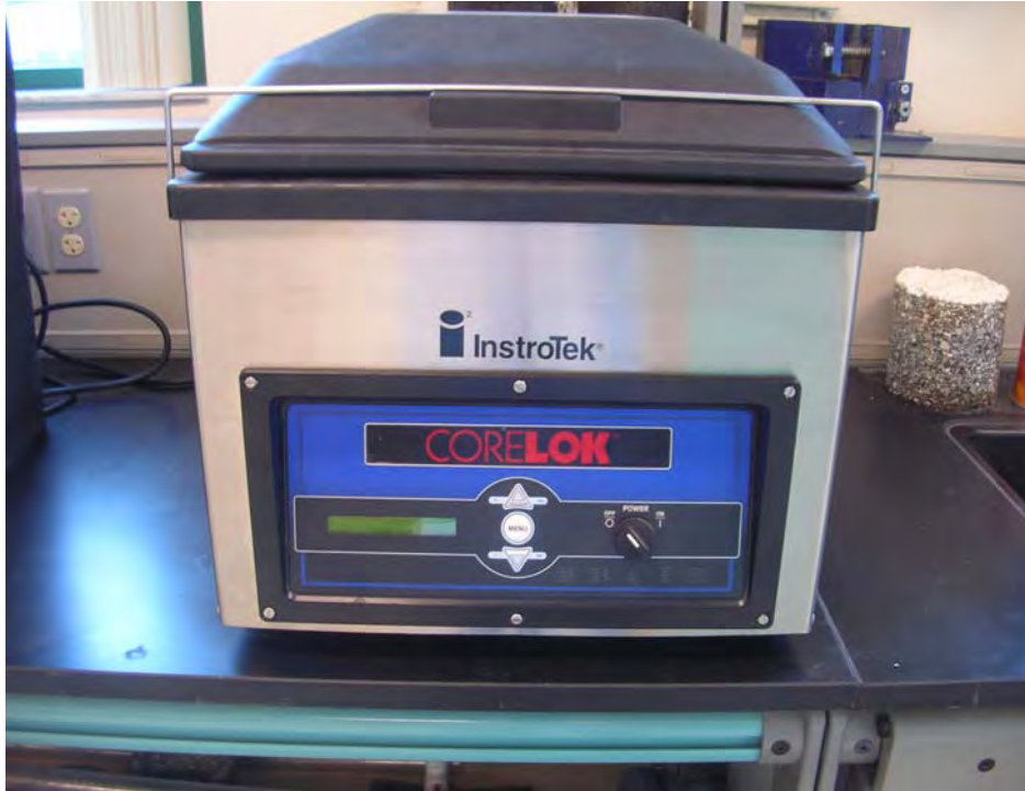
Figure 4-7 Corelok Equipment to Measure Air Void
