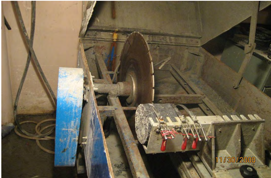
Figure 5-10 Diamond Saw Used for Specimen Slicing
