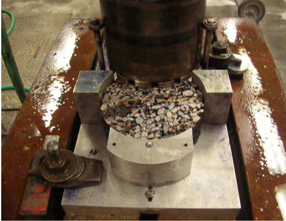
Figure 4-11 Coring Asphalt Mixture Sliced
