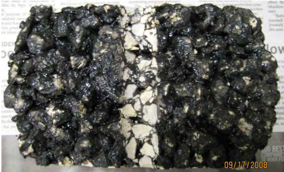
Figure 5-32 Compacted Open-Graded Mixture Surface Without Slicing
