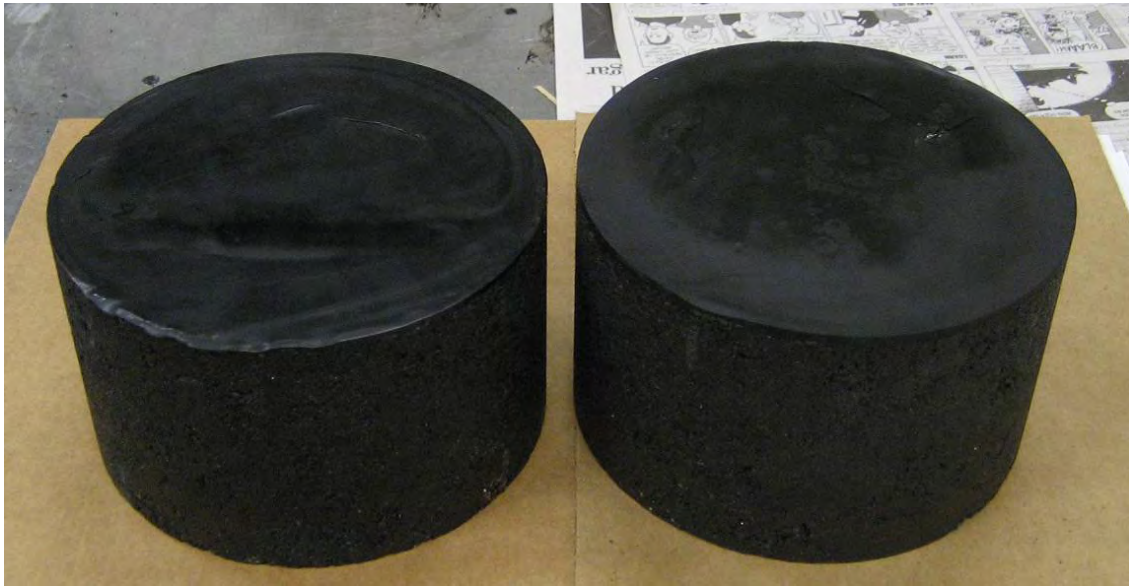
Figure 5-8 Dense-graded Specimens with Applied Tack Coat (left) and Novabond (right)
