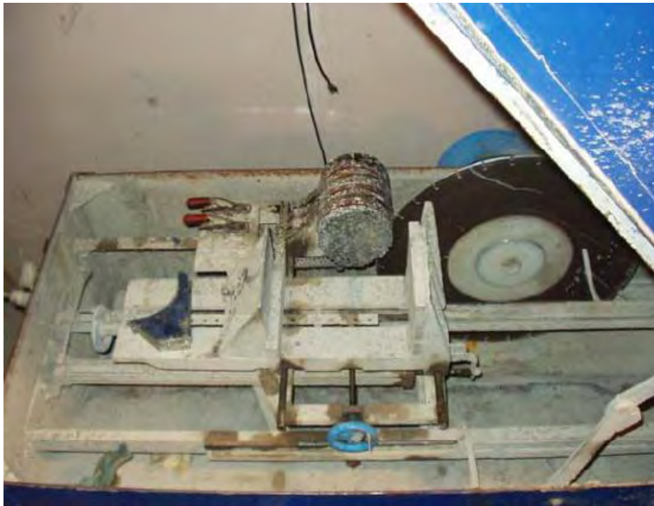
Figure 4-10 Slicing Asphalt Mixture
