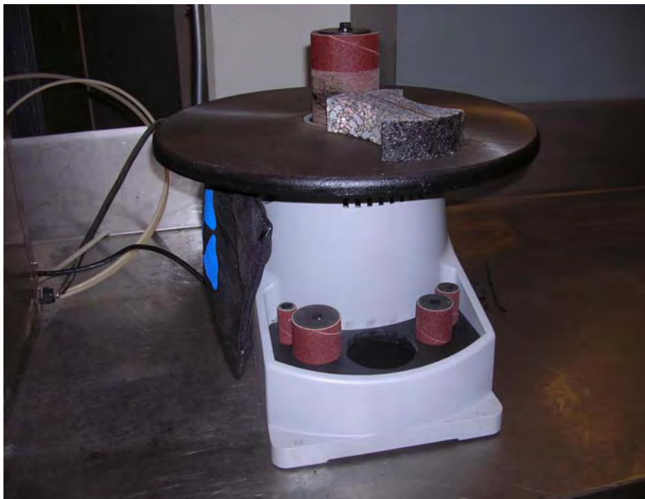
Figure 4-14 Sanding Asphalt Mixture to Eliminate Asphalt Film
