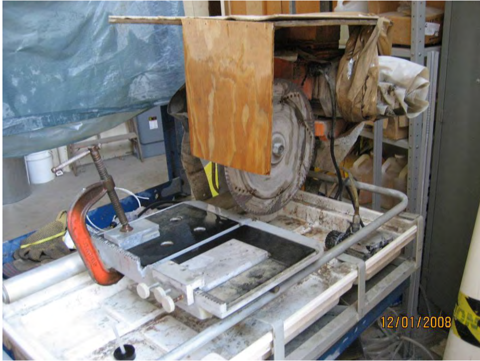
Figure 5-12 Diamond Saw Used for Composite Specimen Straight Cutting
