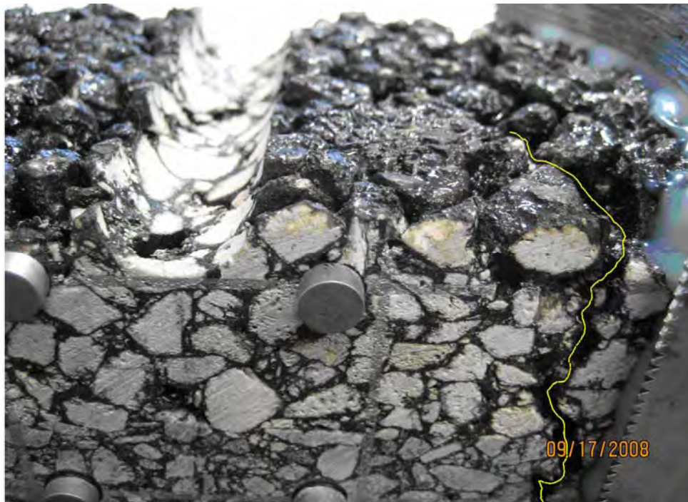
Figure 5-31 Composite Specimen Broke Near the End
