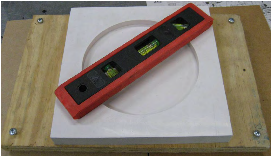
Figure 5-7 Silicone Rubber Mold on Level Shelf
