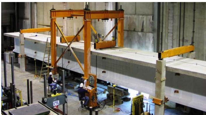
Flexural Strength Test Setup
