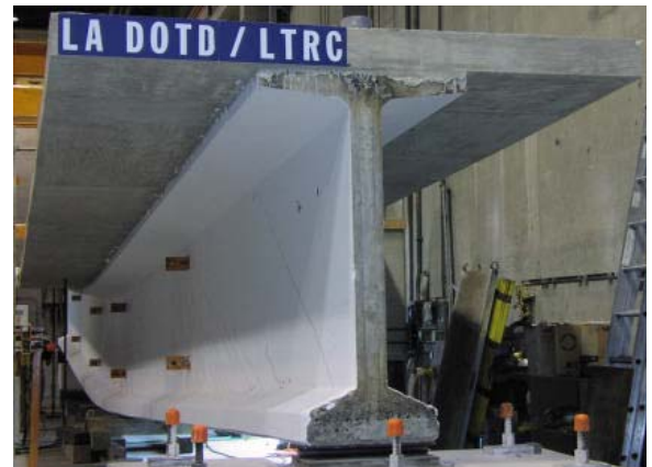
Full-size Bulb-Tee Girder Test
