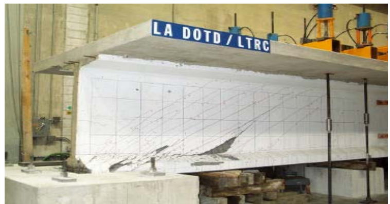
Shear Test at CTL
