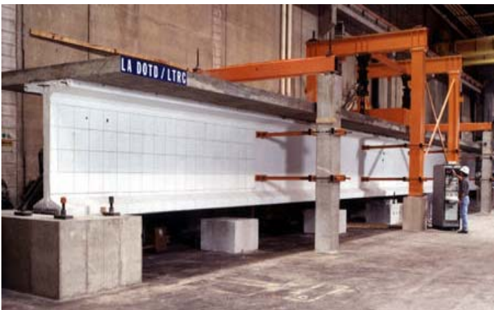
Fatigue Test Setup
