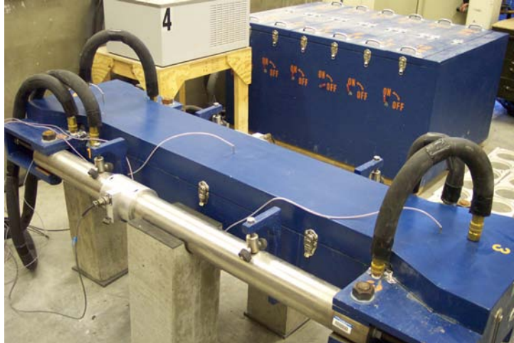
Figure 3.2: Photograph of Rigid Cracking Frame (Whigham 2005)
