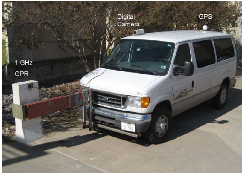
Figure 2. TTI's Latest GPR Vehicle with GPS.
