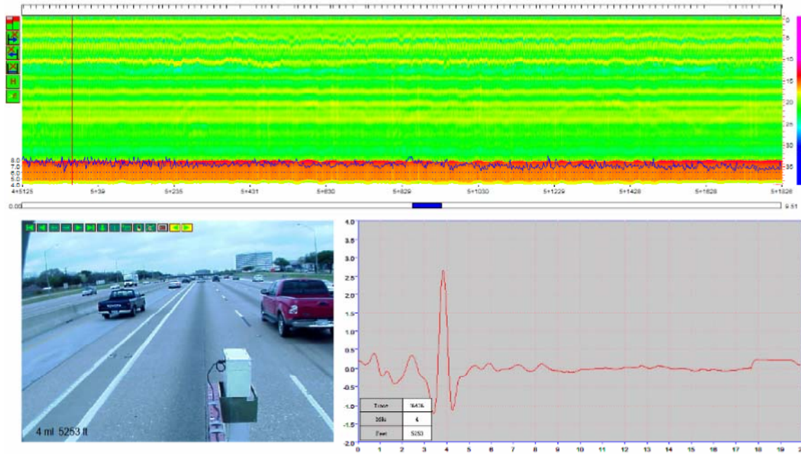
Figure 28. GPR Image of Sampled Section on IH 635.
