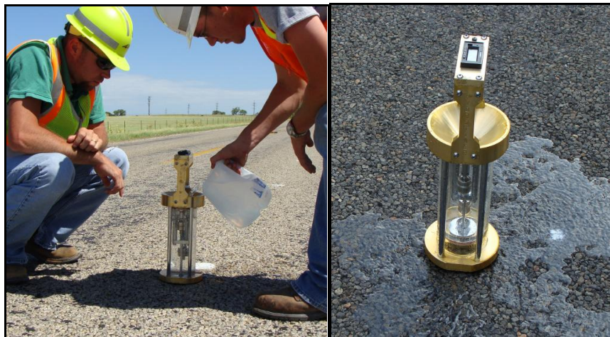
Figure 13. Outflow Meter Test Equipment.
