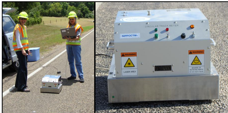
Figure 12. Circular Track Meter Test Equipment.
