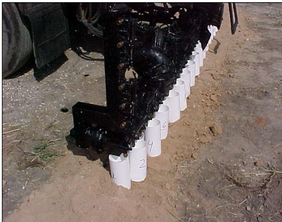
Figure 5. Distributor Calibration (photo provided by R. Walker).
