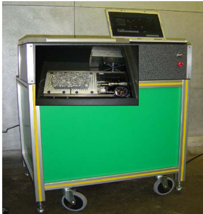
Figure 20. The Overlay Tester and Specimen Setup.
