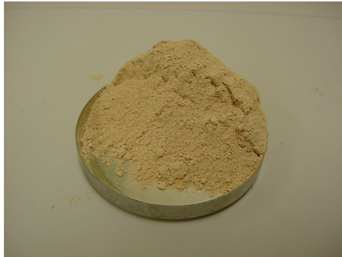
Figure 3.2. A Sample of Oven Dried Crushed Limestone Material
