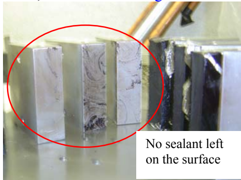
a) Typical adhesive failure
