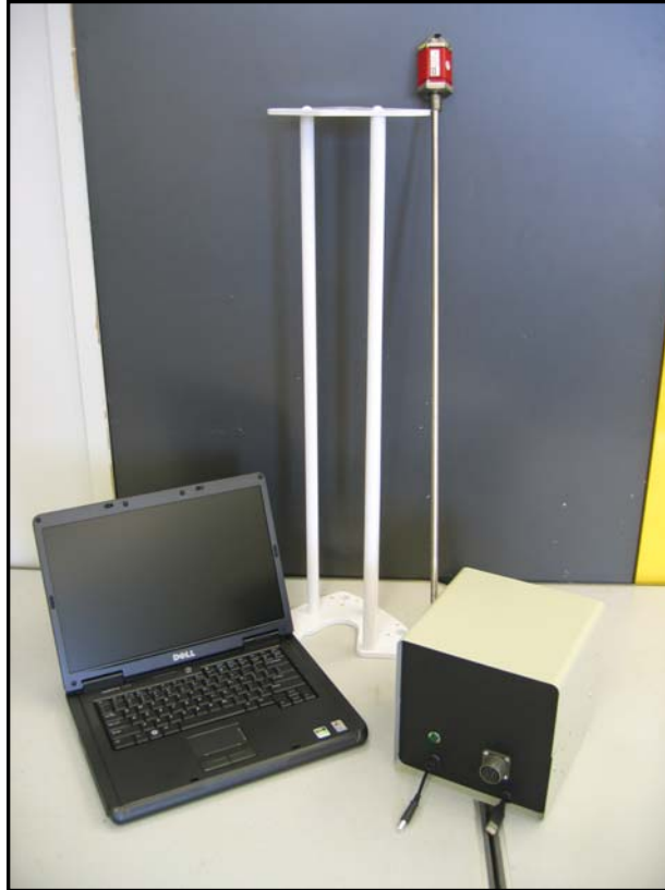
Figure 2.5. Primary Components of the Soil Compactor Analyzer.
