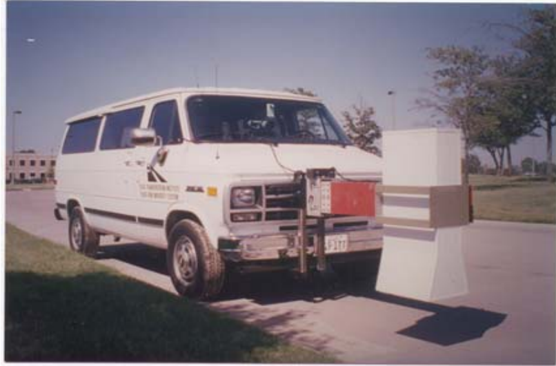
Figure 8-2. TTI GPR Equipment (Scullion, 2006).
