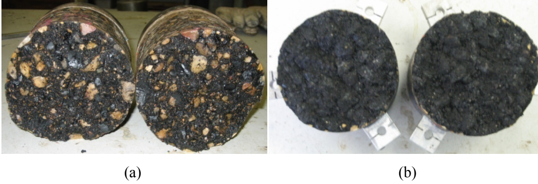
Figure 3-9. Test Specimens after Failure (a) Wet Condition, (b) Dry Condition.
