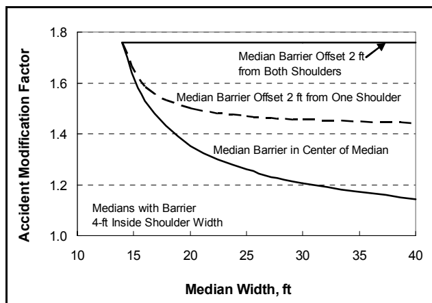
Figure 3-18. Median Width (full barrier) AMF.
