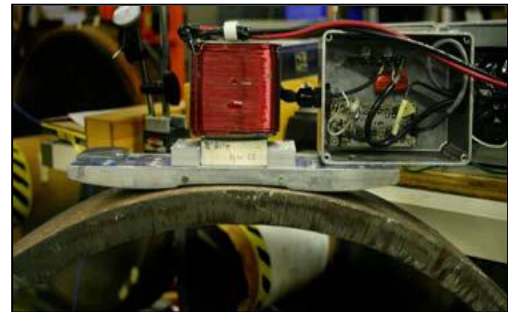
Figure 9: Hand held Crack Detection foot setting on testing loop
