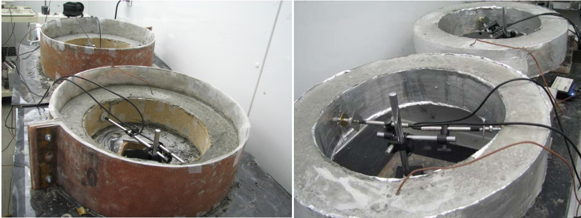
Figure 41: Experimental Setup for free shrinkage measurements from unrestrained ring specimens
