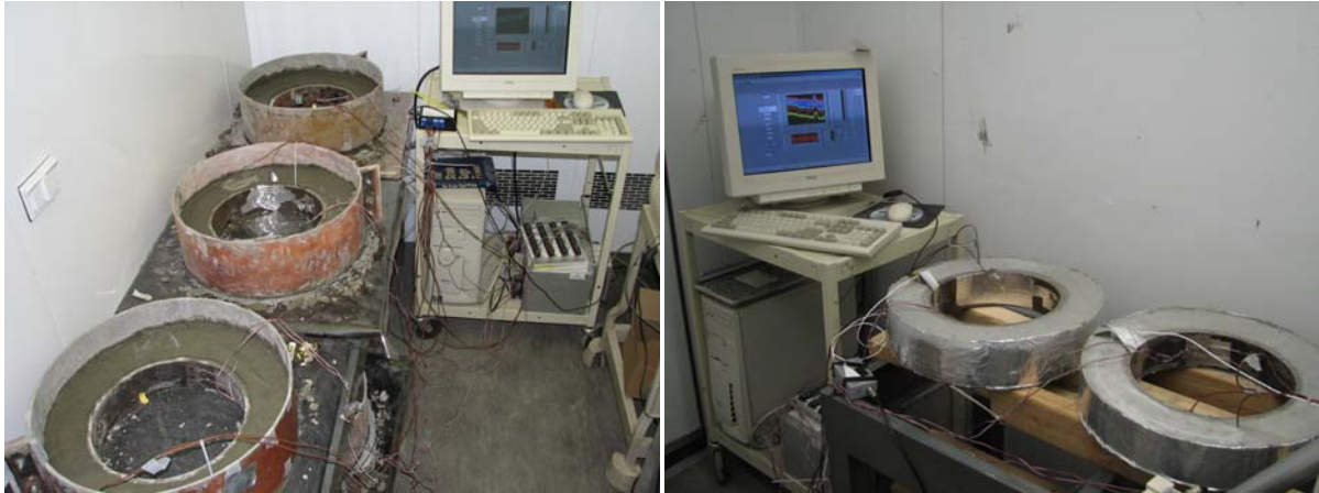
Figure 44: Photographs of experimental setup for restrained shrinkage measurements using ring specimens
