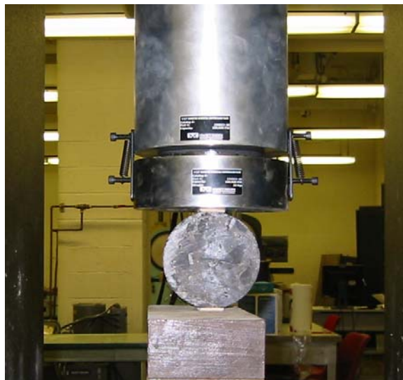
Figure 8: Split tension test setup (ASTM C496 – 96)
