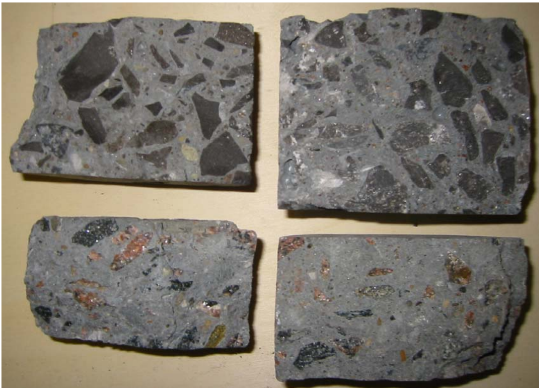
Figure 17: Specimens after performing split-cylinder testing as per ASTM C496 – 96
