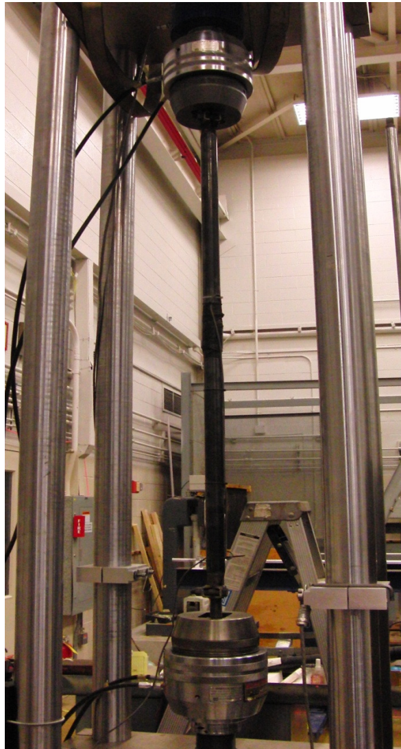
Figure C- 3. Photograph. Tie rod being calibrated in the mechanical test machine.
