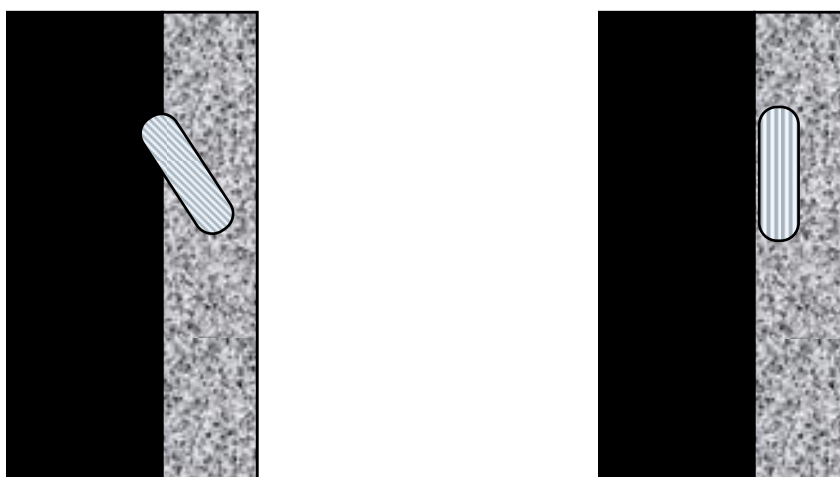
Figure 11. Illustration. Illustrated on the left is a recovery maneuver approaching the pavement edge at an oblique angle. Adjacent is an illustration of a tire grazing the edge of the pavement. Both of these maneuvers were executed during the experiment.
