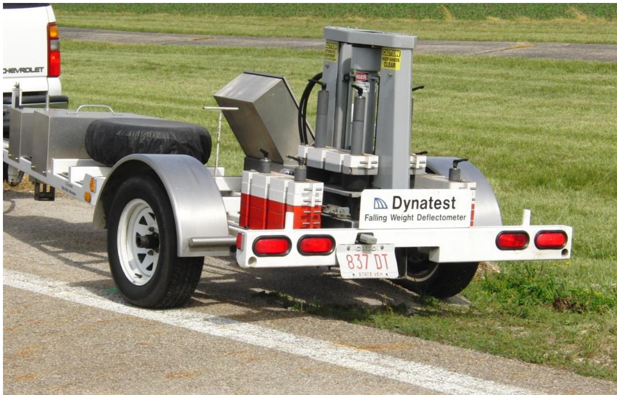
Figure B- 4. Photograph. The falling weight deflectometer.
