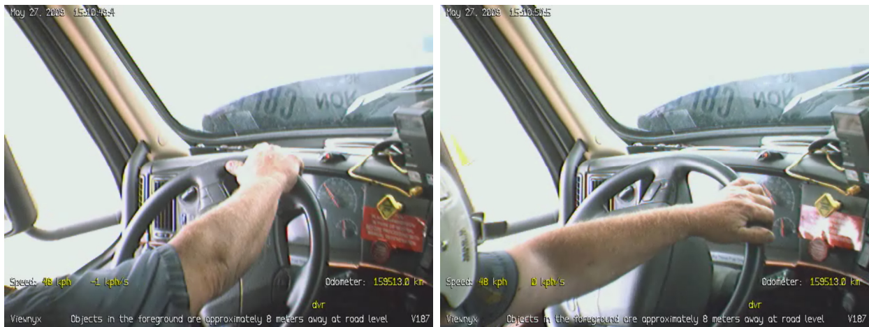
Figure 13. Two photographs. Driver making a recovery maneuver onto the pavement (left) and then countersteering to remain in the original lane (right).
