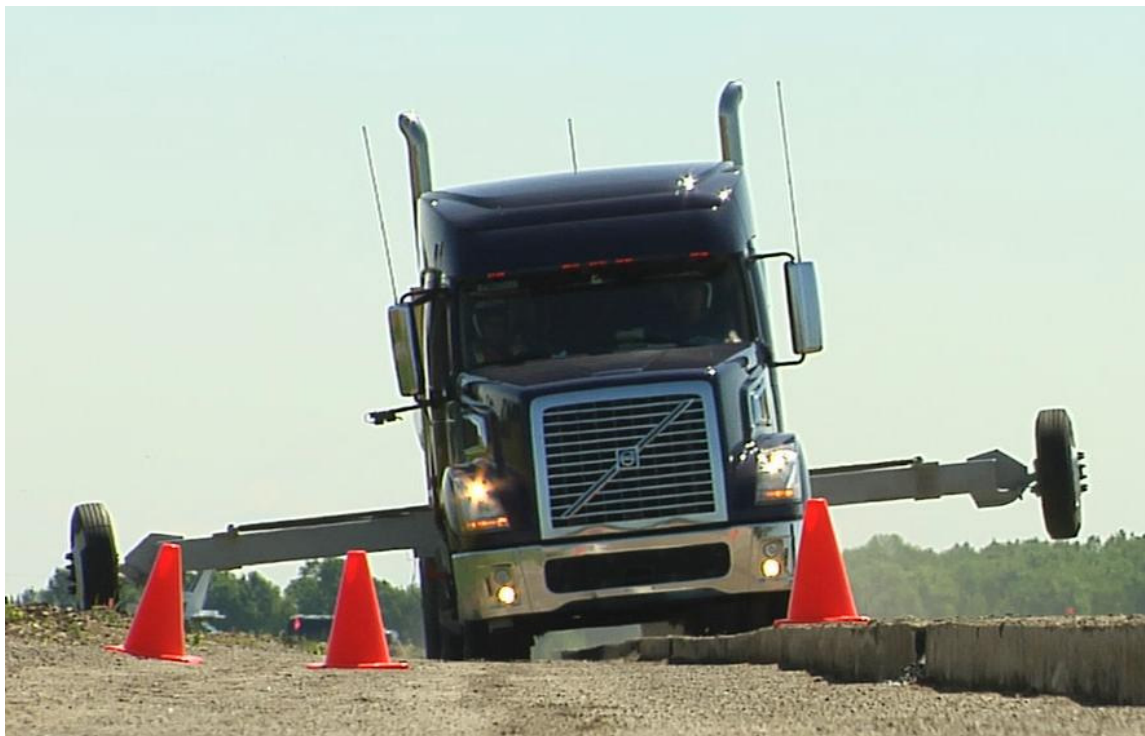
Figure 9. Two photographs. The truck is in a stable straight path with its left tires on the pavement and its right tires in the gravel shoulder.
