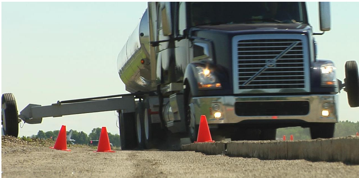
Figure 10. Two photographs. The tractor has climbed the vertical edge, and the trailer will soon follow.
