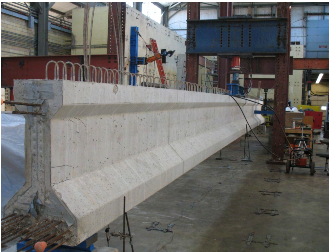
Figure 4-4 Picture of a Type-C Beam Flexural Test Setup
