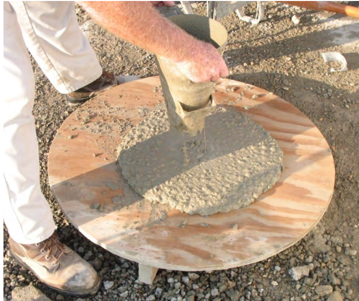
Figure 2-8 Slump Flow Test (TxDOT Research Study 5197)
