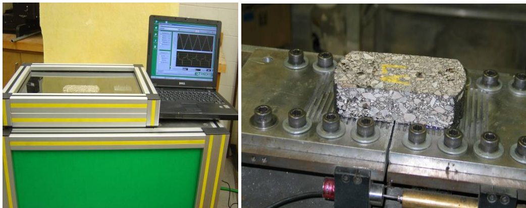
Figure 2. Overlay Tester Equipment and Sample.
