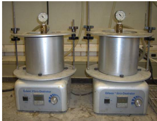
Figure 50. RICE Testing using Metal Vacuum Pycnometer.
