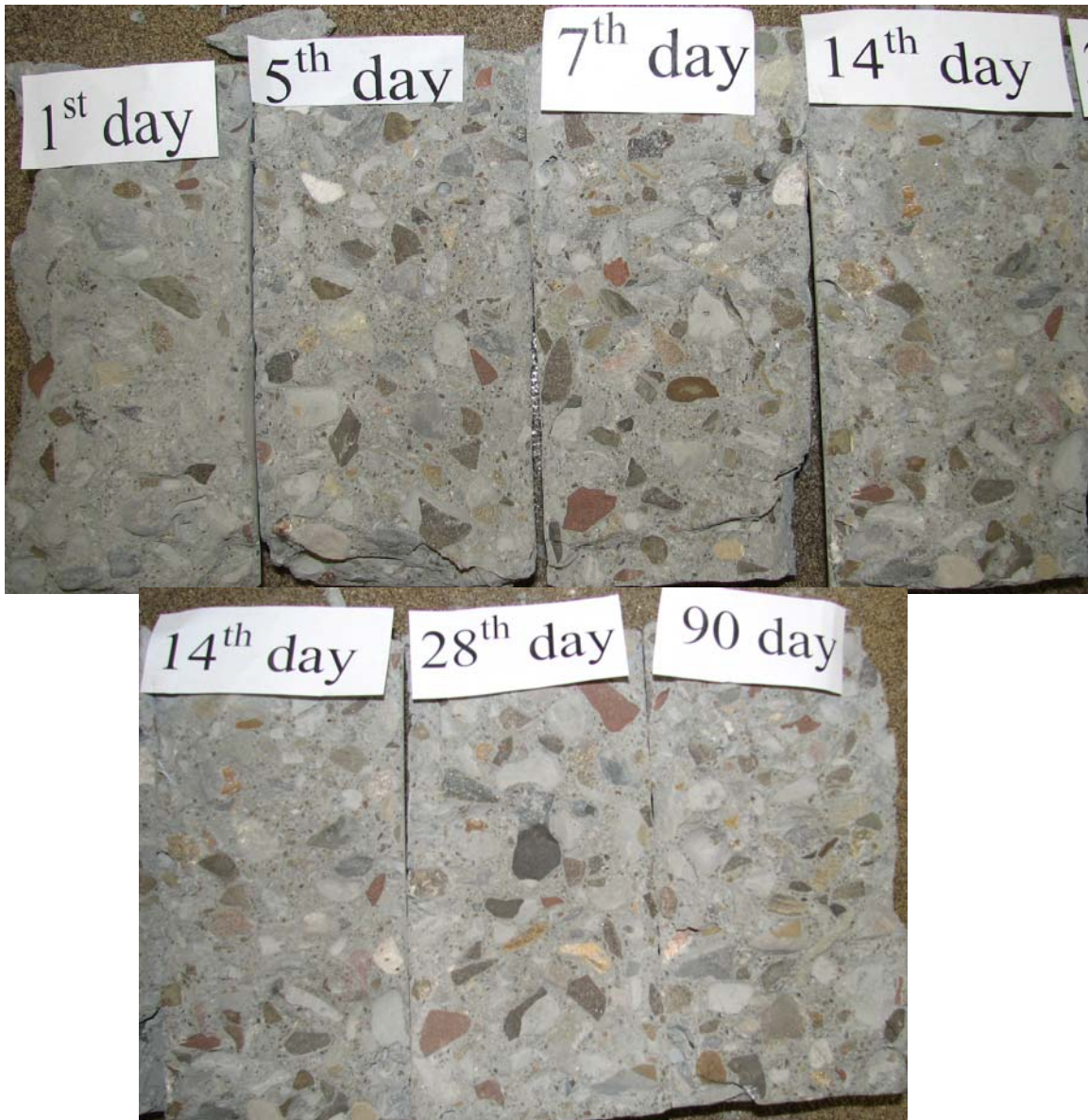
Figure 49: Failure surface of Region 3 specimens at various ages under split cylinder test
