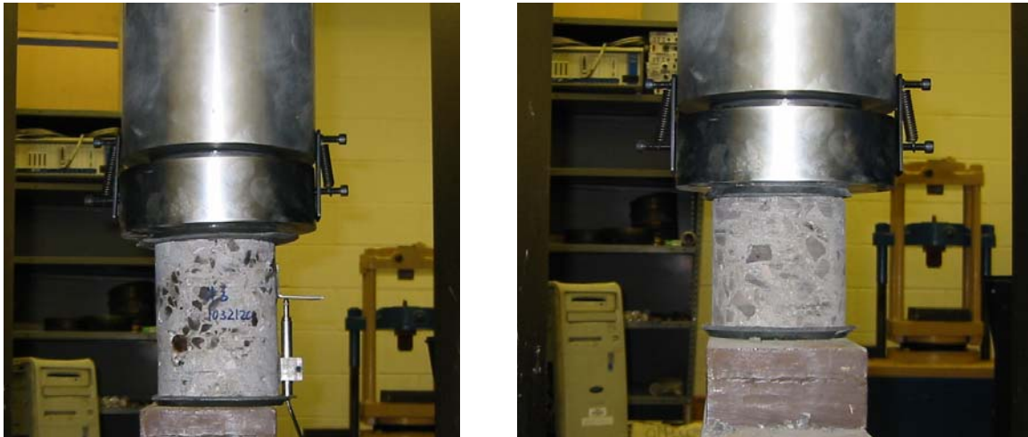
Figure 9: (a) Concrete elasticity modulus set up; (b) ASTM C39/C 39M set up
