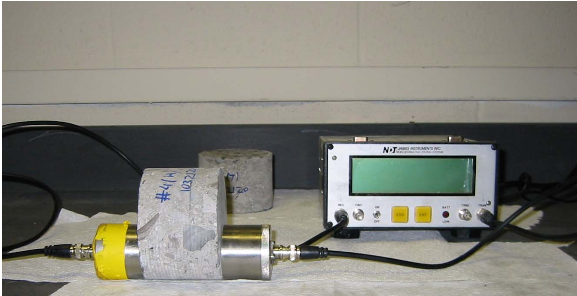
Figure 7: Ultrasonic pulse velocity setup
