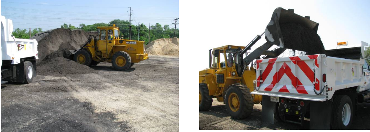
Figure 9. Loader Operation; Material Pickup (left) and Loading Truck (right).
