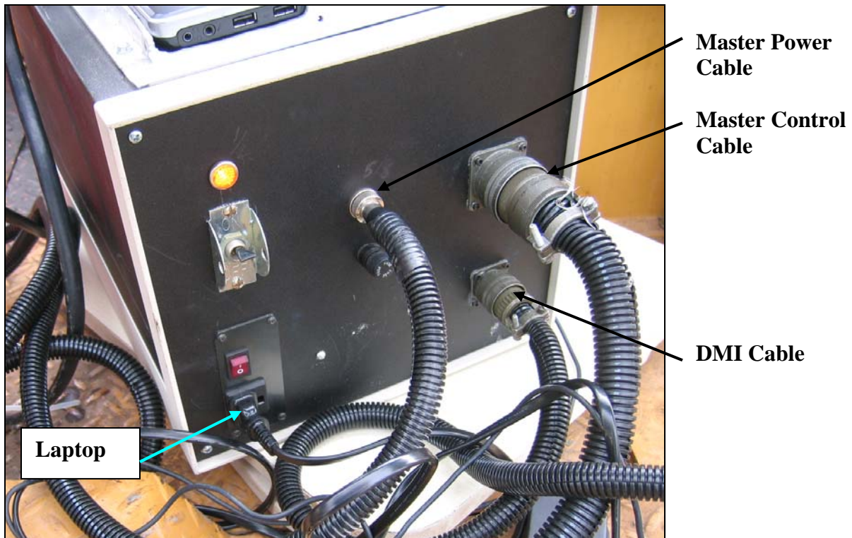
Figure 7. Proper Connections at Master Control Box.
