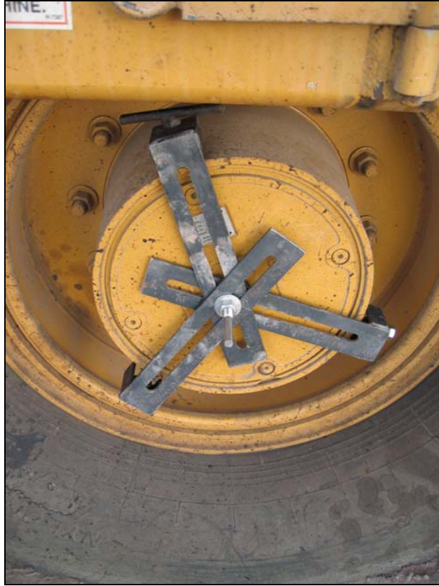
Figure 4. DMI Mount Attached to Paver Wheel Hub.
