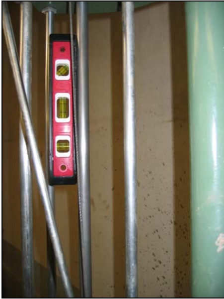
Figure 4. Checking Plumb of Hammer Shaft (Left) and Sensor Rod (Right).
