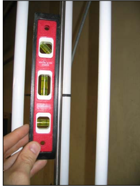
Figure 4. Checking Plumb of Hammer Shaft (Left) and Sensor Rod (Right).
