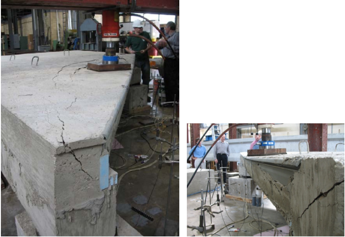
Figure 6.18: Cracking of Specimen 7 at Failure
