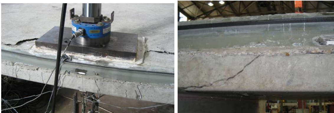
Figure 5.7: Photographs of Specimen 2 after Punching Shear Failure
