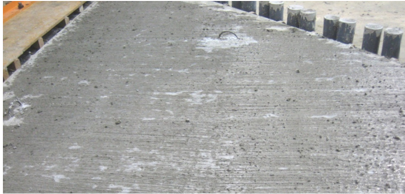
Figure 4.8: Broom Finish Produced in Laboratory
