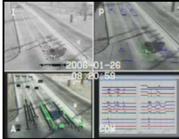
Figure 4.4. Image of shadow from pole and mast arm of crossing street.
