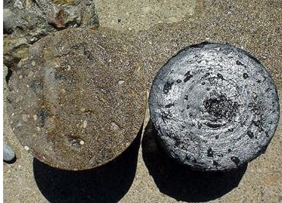
Figure 28. Debonded surface of interlayer fabric (IL 29 Creve Coeur).
