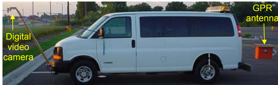
Figure 5. The video integration system (GaVIS) setup.
