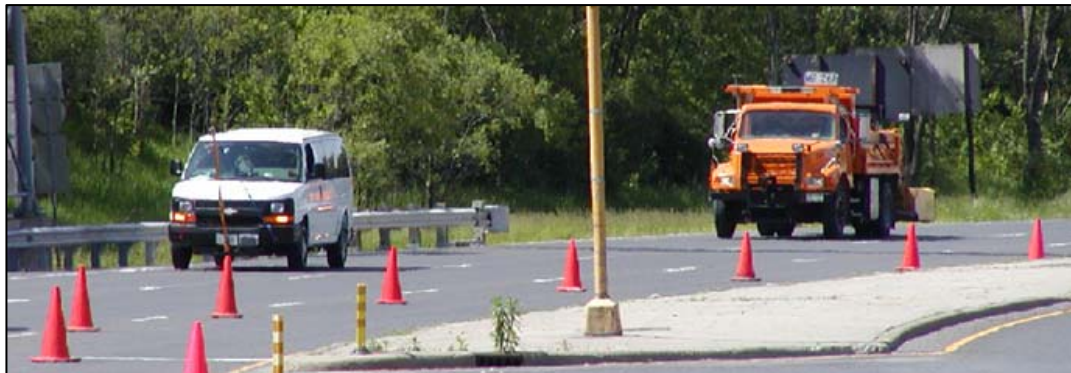
Figure A.13.4. Video and GPR surveys with a moving traffic control.
