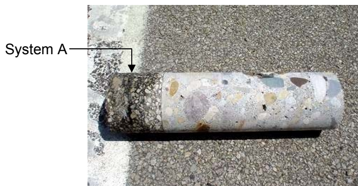
Figure 29. Intact interface shear core from IL 29 Mossville.
