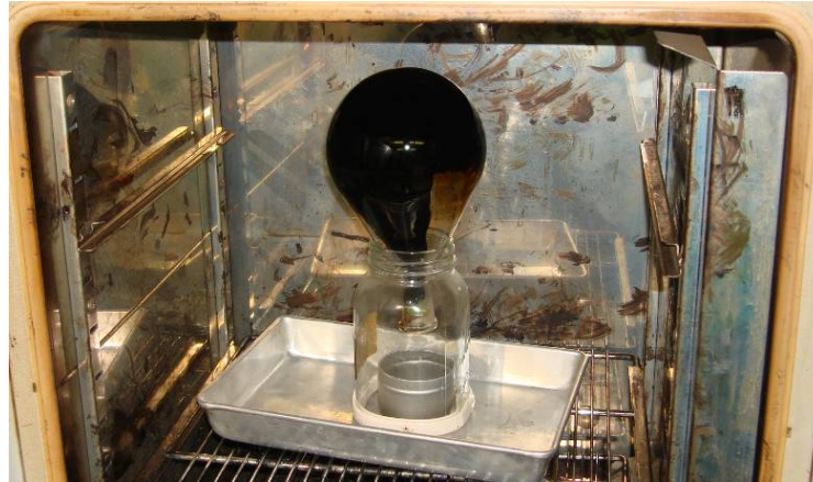
Figure 4. Binder draining from collection flask in oven.
