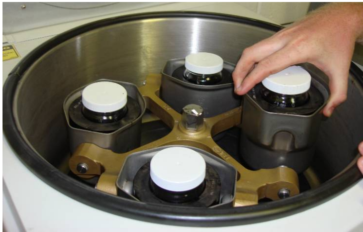
Figure 3. Placing asphalt/solvent solution into centrifuge to remove fines.
