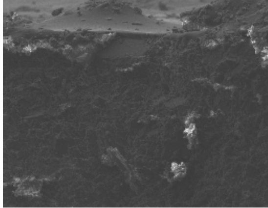
Figure 48. SEM view of PG 64-22 absorption into limestone in SE mode.
