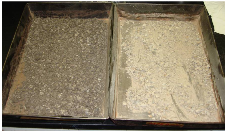
Figure 6. RAP material before (left) and after (right) extraction.
