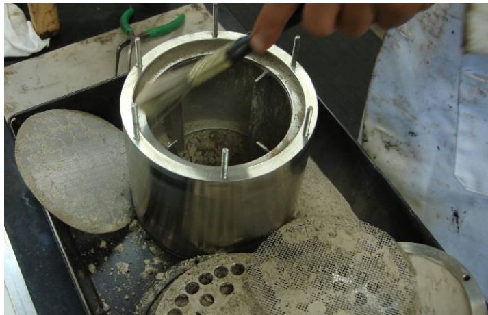
Figure 5. Brushing the extraction vessel clean of fine material.
