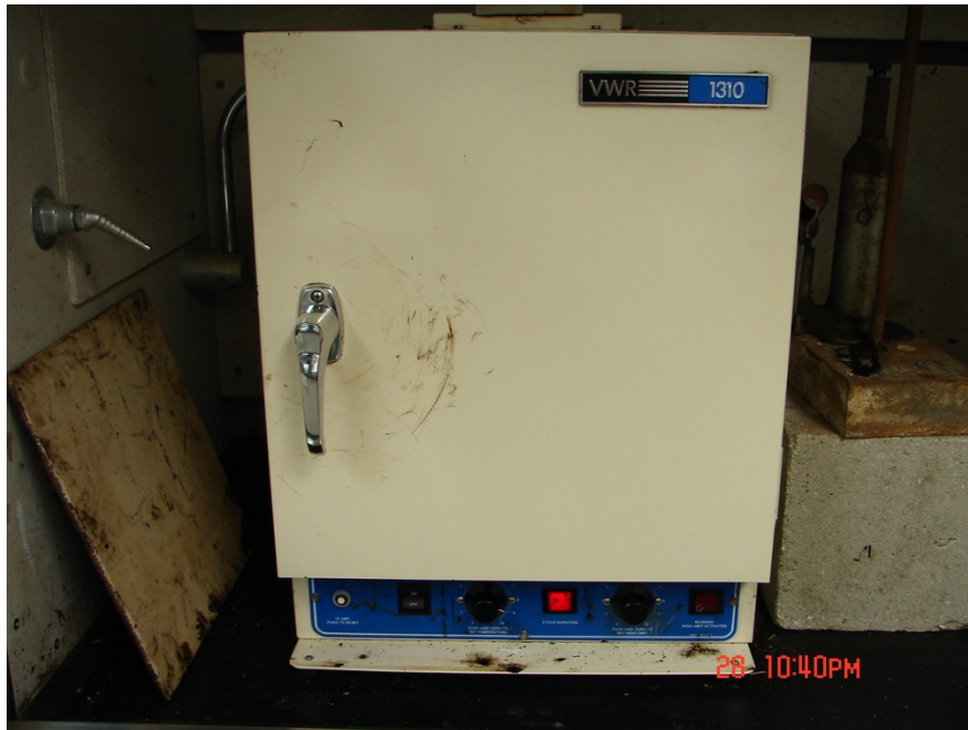
Step 3: Heat a conventional laboratory oven B to 50°C blow below the recommended pouring temperature.
