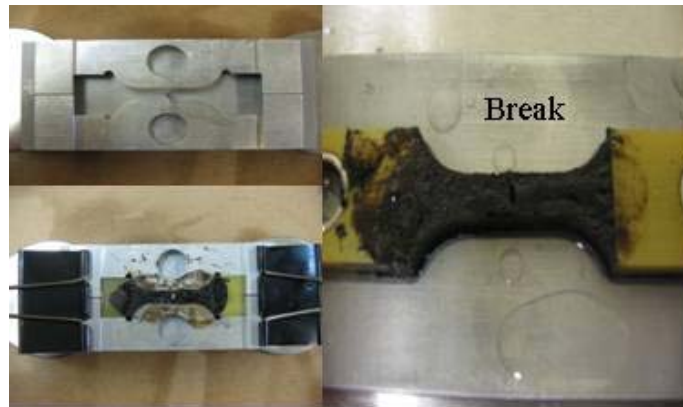
Figure 6 Mold for preparing middle centered notched specimen of crack sealants
