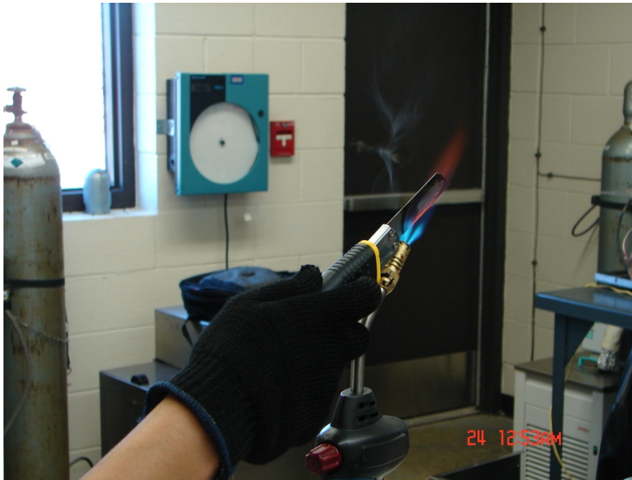
Step 12: Use a propane blow torch to heat a cutting knife.
