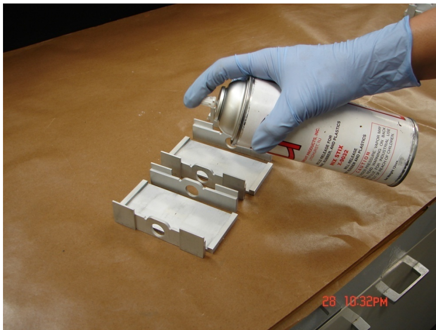
Step 4: Spray release agent (Nix Stix X-9032 from Dwight Products) onto test sample mold.
