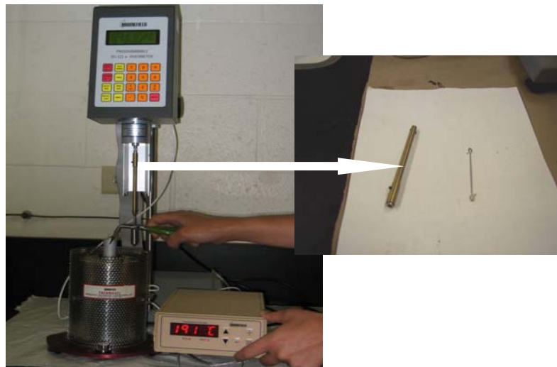
Figure 1. Brookfield Thermosel system, rigid and a new rod used in viscosity testing of crack sealants and asphalt binder, respectively
