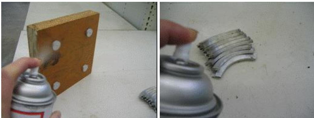
Figure C-4. Spray release agent on the plugs and the molds
