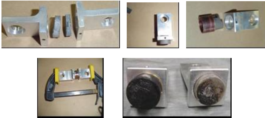
Figure 4. Adhesion test using split-mold and sealant failure to covering end pieces (lower right)
