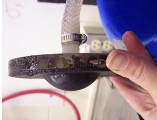
Figure 15. The first trial of the blister test: annular plate covered with sealant and the connector hose
