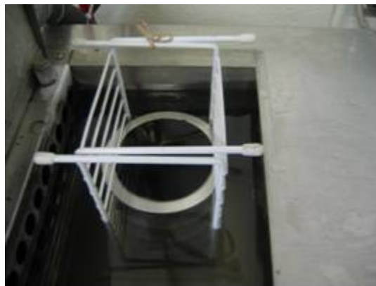
Figure C-16. Condition the specimens in the bath for 20 minutes
