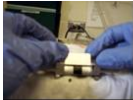
Figure B-15. Remove the mold while keeping the two end pieces in place
