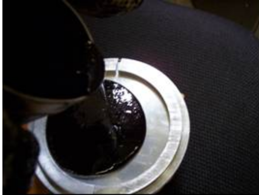
Figure C-8. Mix sealant thoroughly and pour on center top of the plug and let it flow to fill the mold
