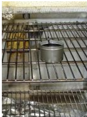
Figure B-1. Heat 35 gram of homogenized sealant at recommended pouring temperature for 30 minutes
