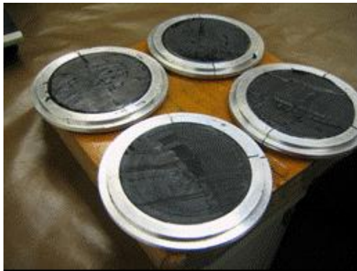
Figure C-9. Let the sealant set for one hour at room temperature
