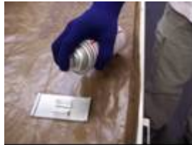
Figure B-3. Spray release agent on the mold
