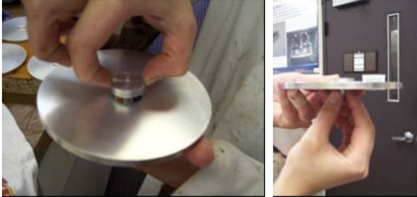
Figure C-5. Place the plug on the annular plate, and pull it from underneath the plate until it fits in the orifice and the film edges sits on the plate
