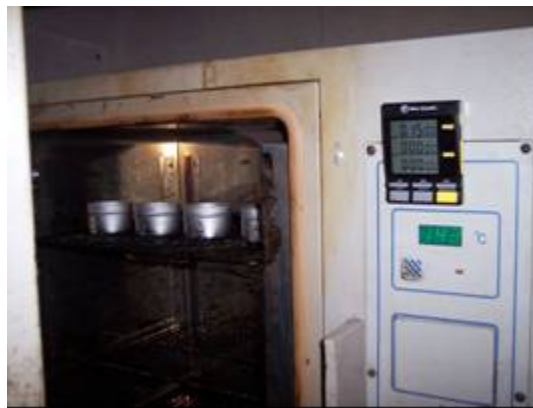
Figure C-1. Heat four cans of 80g homogenized sealant for 15 minutes at the recommended pouring temperature
