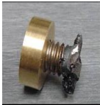
Figure 3. Anchorage used in adhesion test
