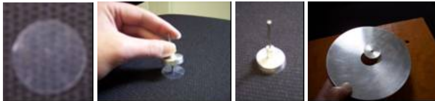
Figure 20. Aligning the FEP film on the plug and installing the plug in the orifice
