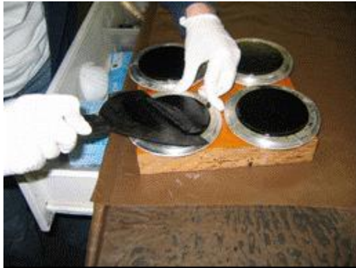
Figure C-10. Trim the extra sealant away with a heated potty knife
