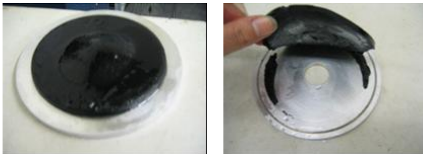
Figure C-24. Remove the sample and examine if the failure type was adhesive in which sealant film separates from the plate
