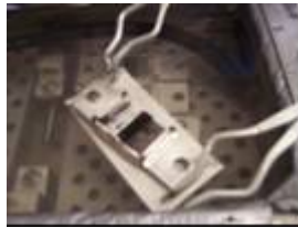
Figure B-9. Grab the base plate with two tangs and place it in cooling bath
