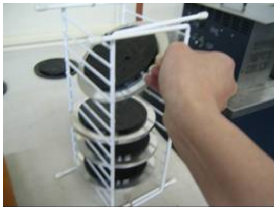
Figure C-13. Place the plated on the rack; allow enough clearance between each two specimens
