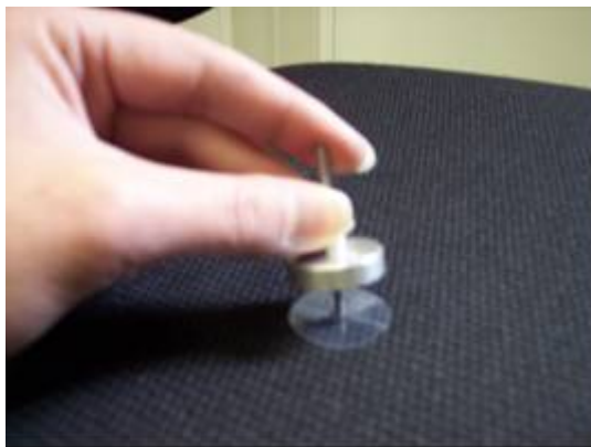
Figure C-3. Peel the transparent film, and place it on a flat surface with adhesive side up, place the pin on its center and let the plug slide through the pin to the film
