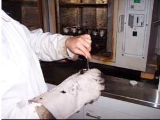
Figure C-2. Remove the can, mix the sealant thoroughly and place it back in the oven for another 15 minutes
