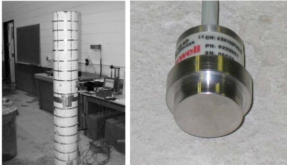
Figure 11. PVC column (left) and pressure sensor (right) used in laboratory tests [4].
