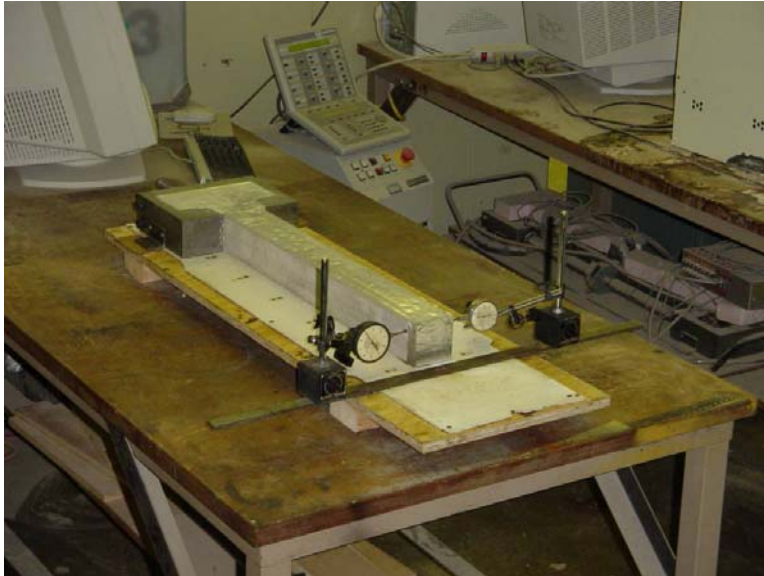
Figure 21. Differential shrinkage test for validation of ICON 3-D finite element model [5].
