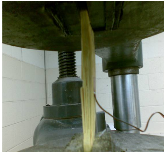
Figure 4.4: Fiber Composite Tubular Section Coupon after Testing
