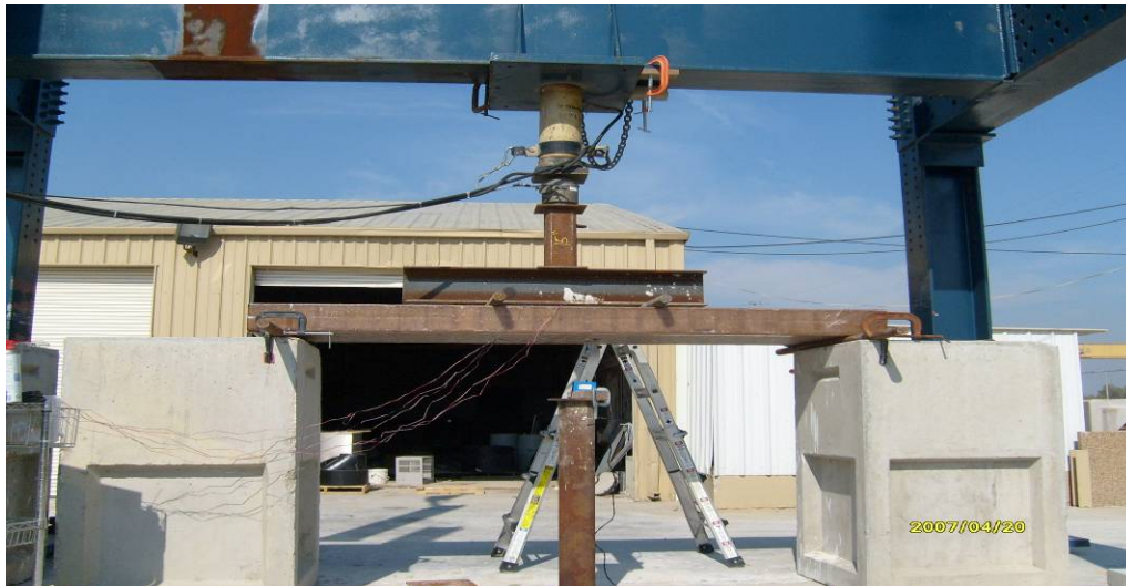
Figure 4.5: Four Point Bending Test
