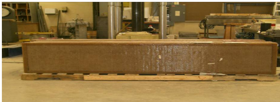
Figure 3.1: Fiber Composite Bridge Deck of Size 2 feet x 8 feet
