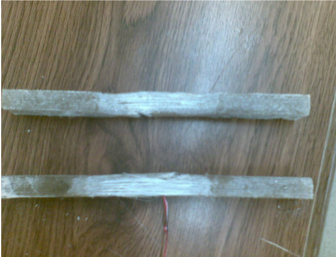
Figure 4.3: Fiber Composite Deck Coupon after Testing
