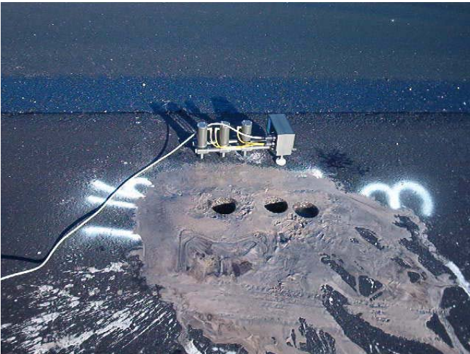
Figure N.5 – PSPA Collecting on Core Location at Site 1
