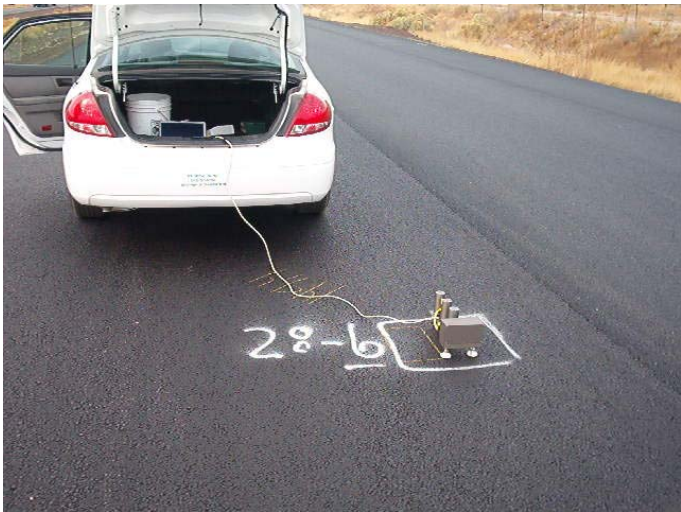
Figure N.23 – PSPA Testing on Core Location of Site 8
