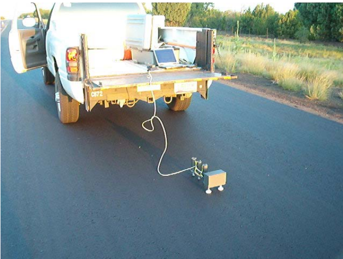
Figure N.8 – PSPA Collecting on Site 2
