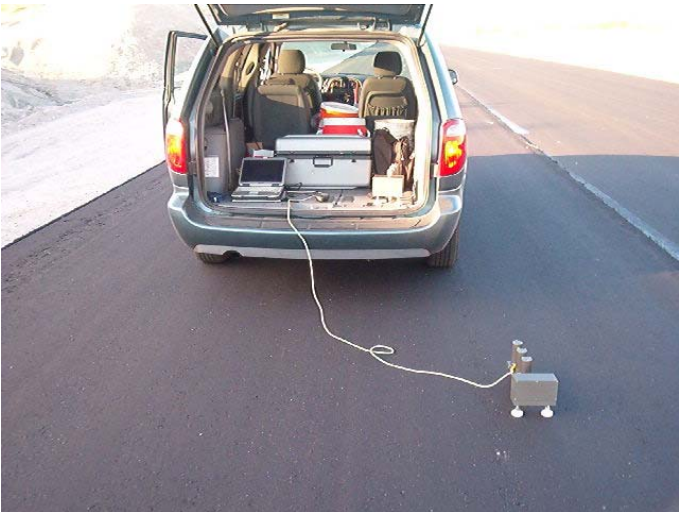
Figure N.4 – PSPA Collecting Information on Site 1
