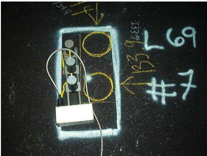
Figure N.29 – PSPA Testing on Core Location of Site 10
