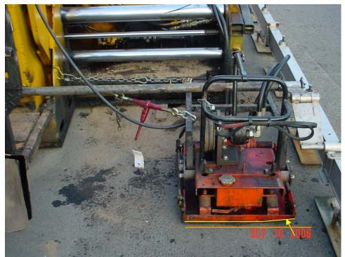
Figure #3 Wedge Compaction Device and Setup
