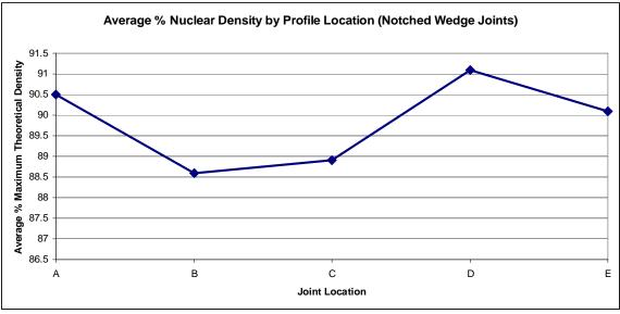
Figure #11 – Notched Wedge Average % Corrected Nuclear Density by Profile Location
