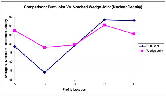
Figure 15. Butt Joint Vs. Notched Wedge Joint (Nuclear Density)
