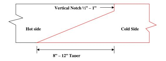
Figure #4 Notched Wedge Joint Diagram
