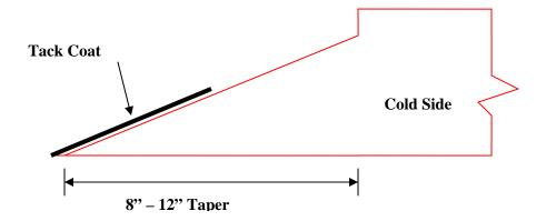
Figure #7 Tack Coat On Bottom Half of Wedge
