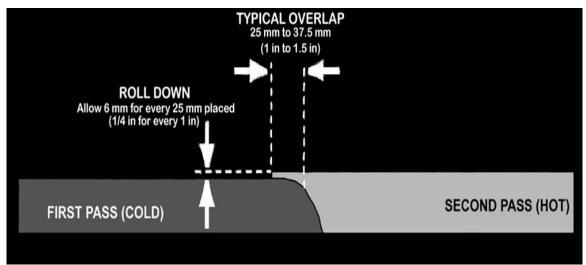
**Figure 1. Typical Butt Joint Construction Protocol**
