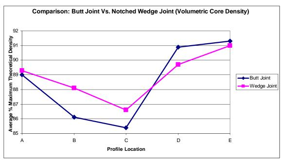
Figure 16. Butt Joint Vs. Notched Wedge Joint (Core Density)
