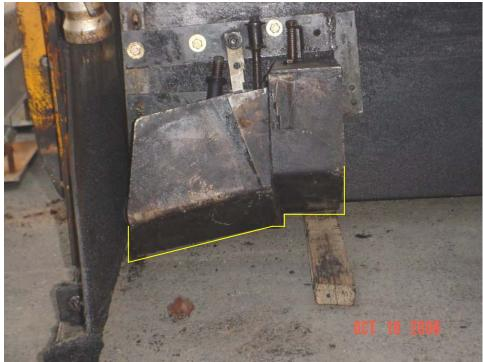
Figure #2 Notched Wedge Forming Device
