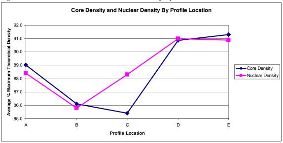
Figure #14. Core and Corrected Nuclear Density by Profile Location
