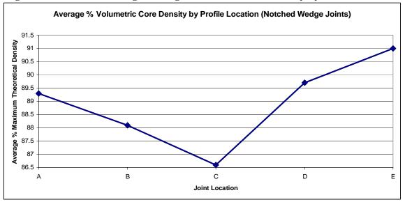
A = 1 foot cold side B = 6 inches cold side C = joint location D = 4 inches hot side E = 1 foot hot side
