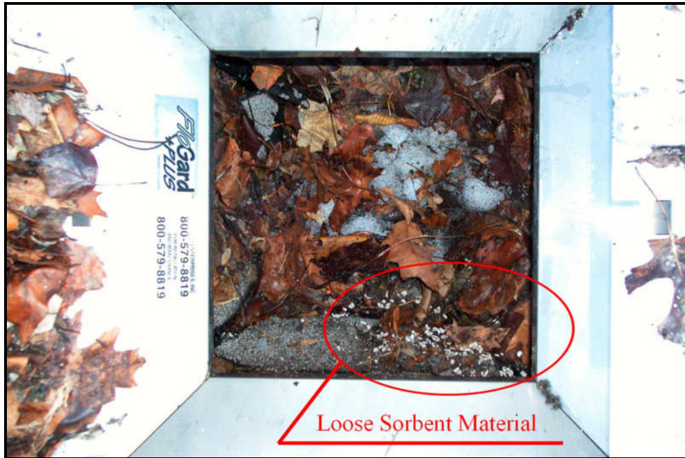
Figure 32: FloGard® +PLUS - Loose absorbent material
