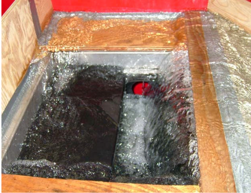
Figure 11: Hydro-Kleen™ insert tested with flow rate of 300 liters per minute.
