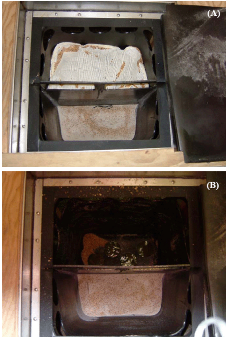
Figure10: Hydro-Kleen™ insert (A) after testing medium flow, high concentration (fully drained). Hydro-Kleen™ insert (B) with the pillows removed (water did not drain out of first chamber).
