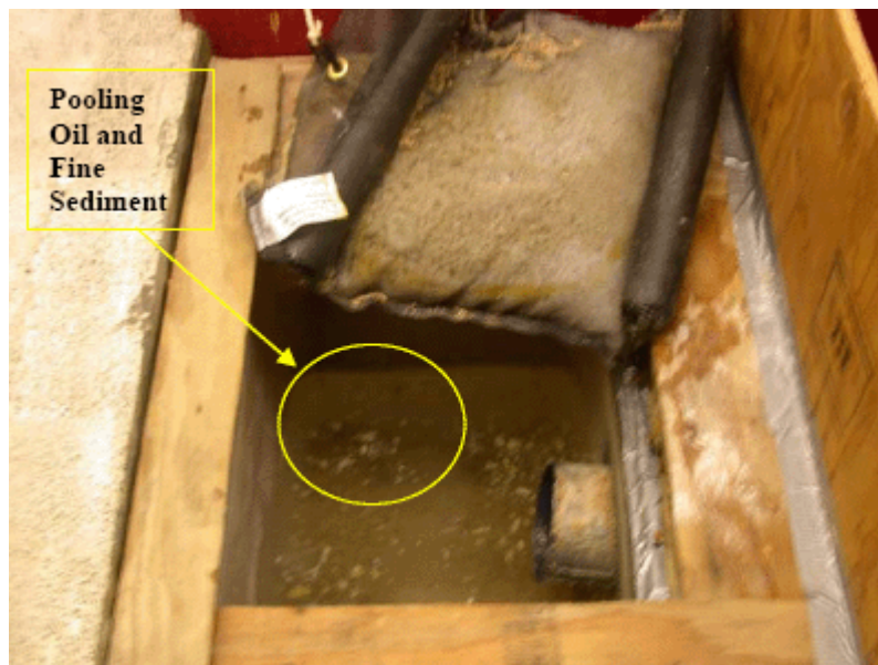
Figure 17: The catch basin with the Passive Skimmer removed after the test.
