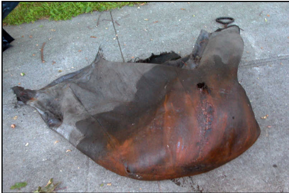
Figure 31: Silsack® - Hole in the geotextile fabric
