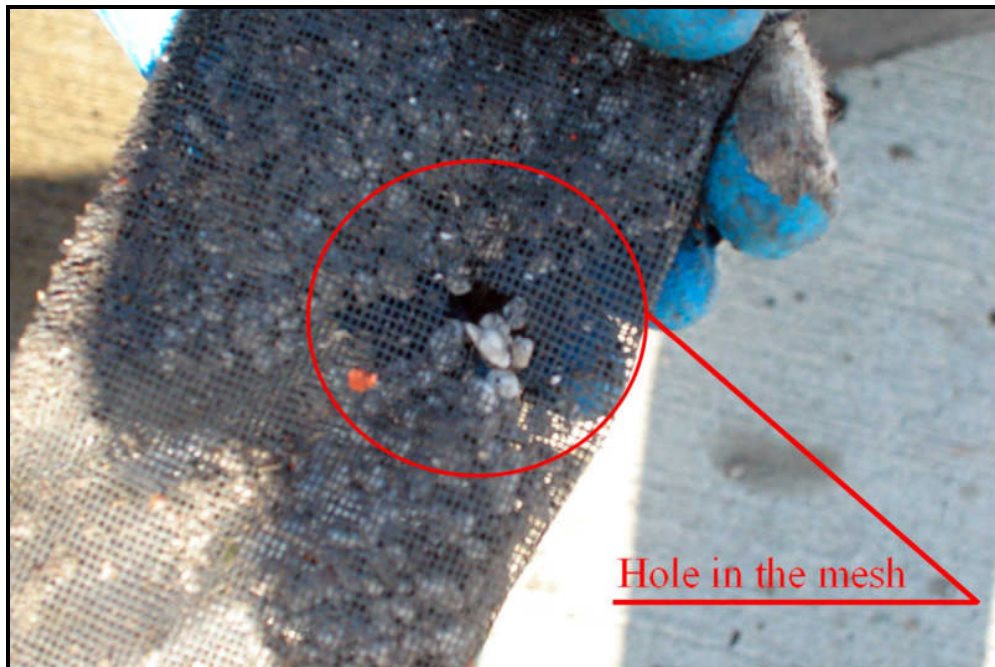
Figure 33: FloGard® +PLUS – Hole in the mesh that holds the absorbent material
