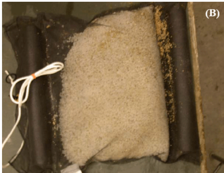
Figure 14: Passive Skimmer: (A) unused and (B) used with medium flow, high concentration.
