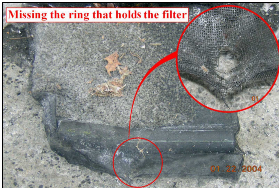
Figure 37: Passive Skimmer™, missing the ring that allows the tying of the filter
