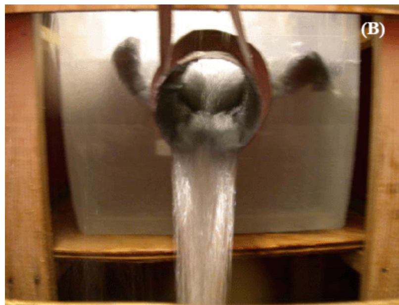
Figure 15: Passive Skimmer at 150 liters per minute: (A) view from above and (B) side of simulator.
