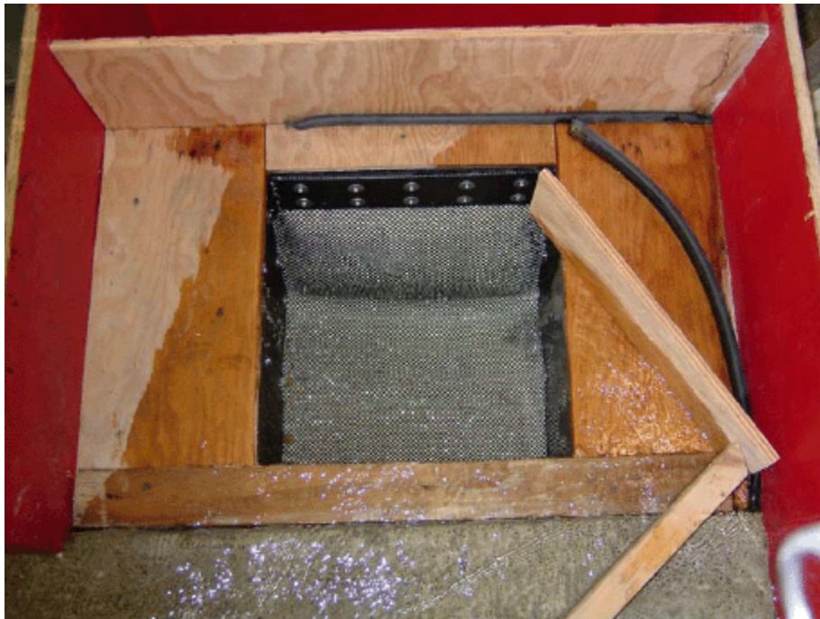
Figure 12: Ultra-Urban® insert (top and bottom) tested with clean water, flow rate of 150 l/min.
