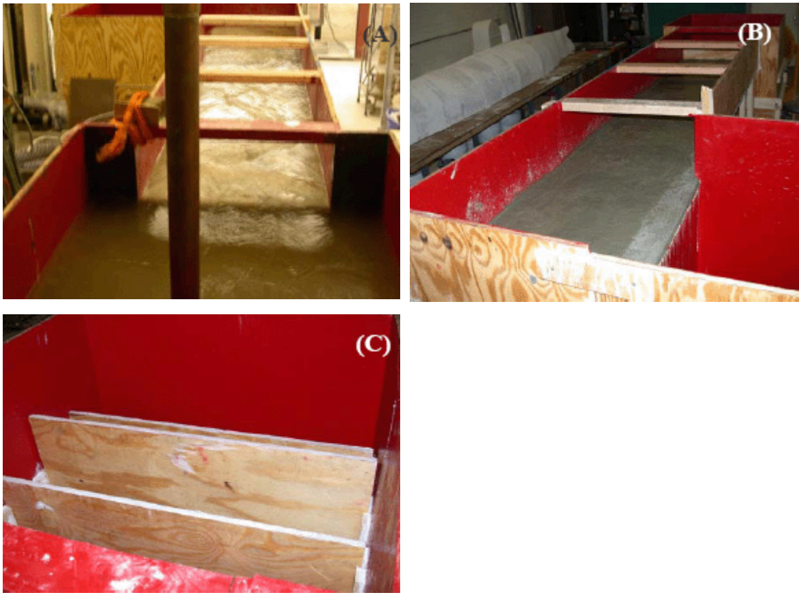
Figure 5: Simulator photographs: a) spillway view from stilling chamber (no baffles), b) cement-lined spillway view from catch basin, c) baffle setup in stilling chamber.
