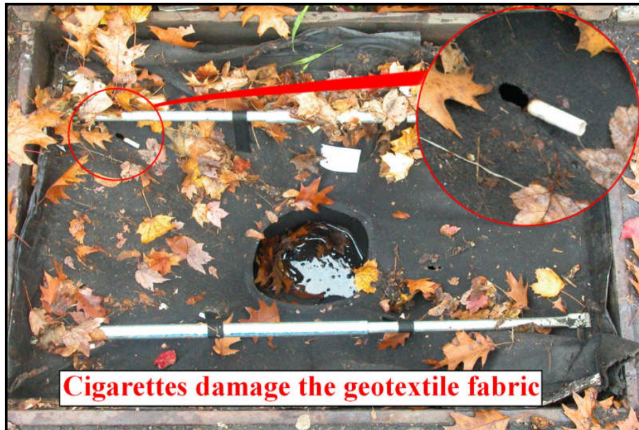
Figure34: Stream Guard™ filter, holes in the fabric caused by lit cigarettes
