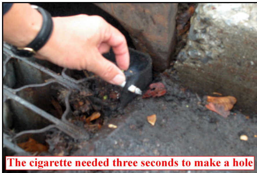
Figure 35: Stream Guard™ – Test performed with a lit cigarette on the fabric
