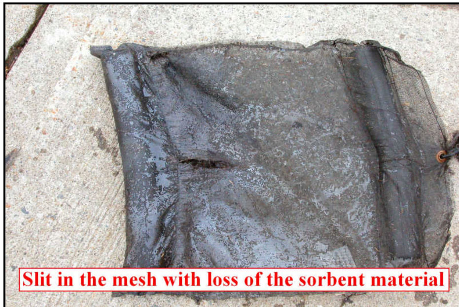
Figure 36: Passive Skimmer™, slit in the mesh with loss of absorbent material
