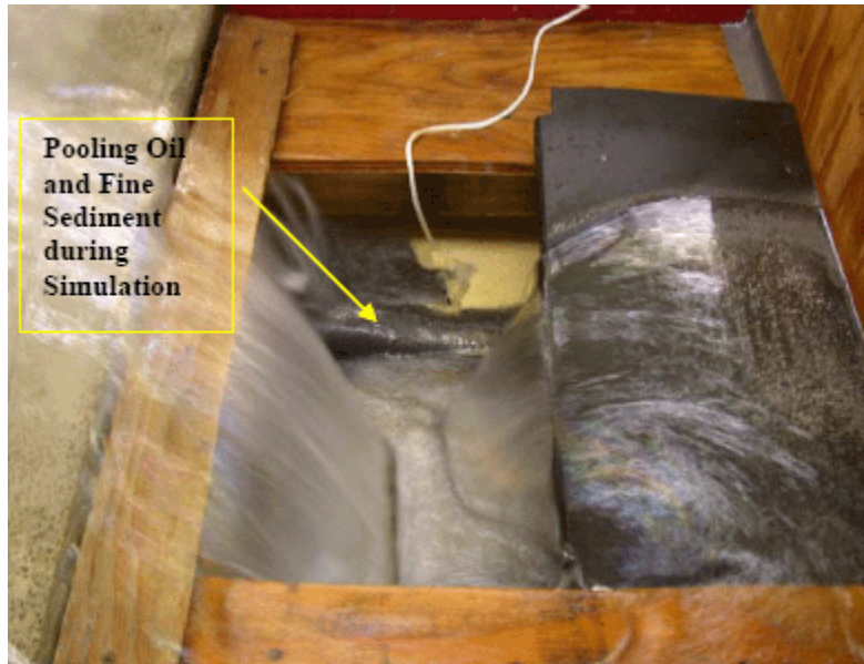
Figure 16: Passive Skimmer during high flow rate, high concentration test after 40 minutes.
