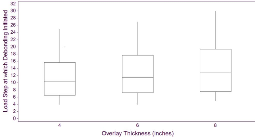
Figure 4.18: Effect of the overlay's thickness on debonding initiation
