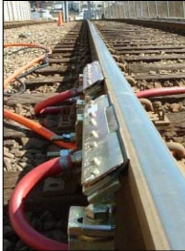
Figure 8.12: Trackside Friction Modifier Applicator Source: Portec Rail
