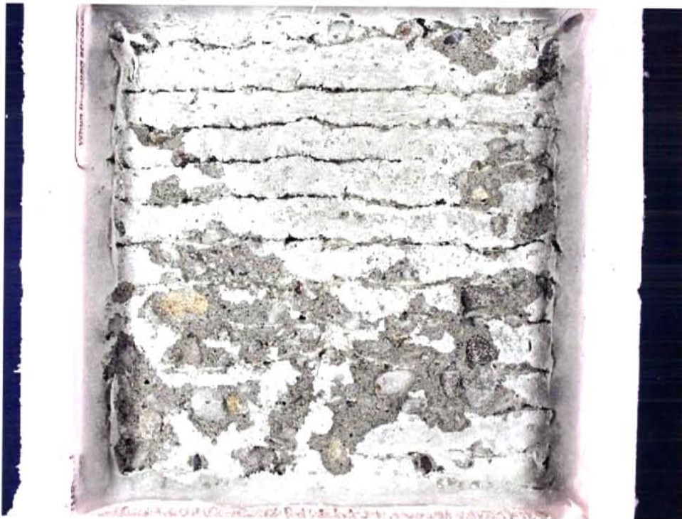
Fig 2 – Deicer Scaling Resistance–Mix 1 (SF) Sample B before testing (above) and after testing (below)
