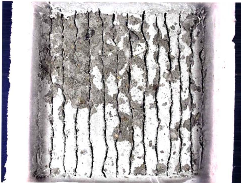
Fig 3 – Deicer Scaling Resistance–Mix 2 (C) Sample A before testing (above) and after testing (below)
