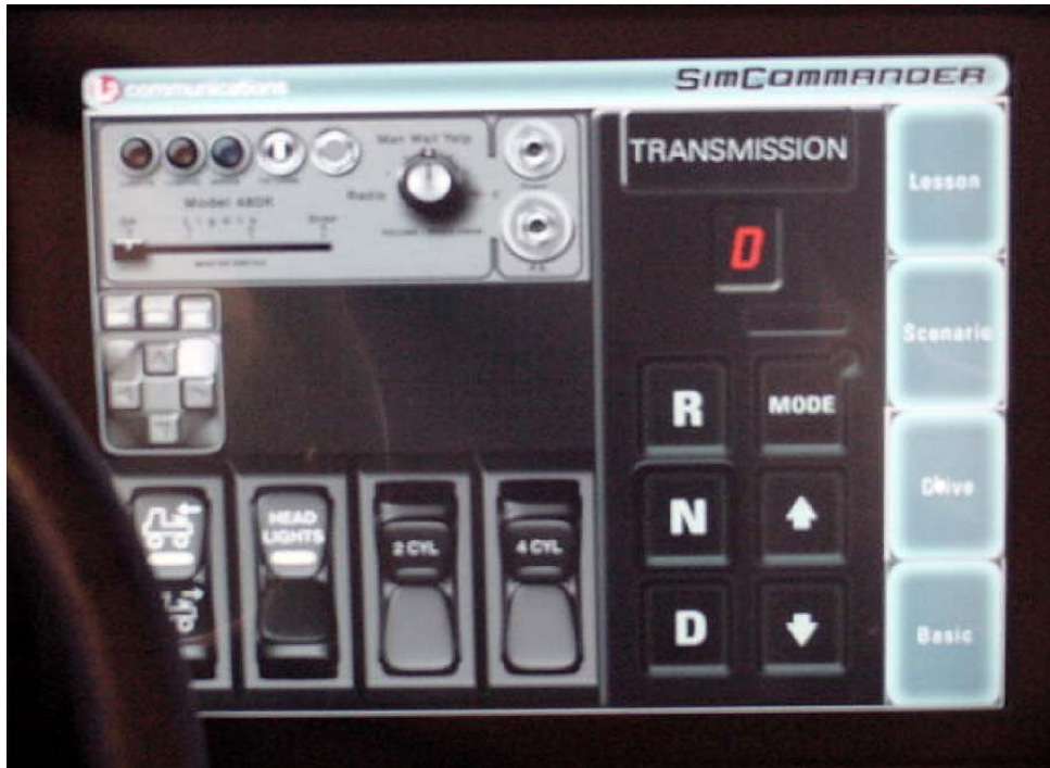
Figure 6. Simulator Display — Automatic Transmission
