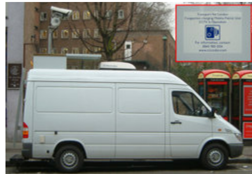
Figure 5 - A mobile enforcement vehicle is used to photograph number plates within the London congestion charging zone. Photo provided by Transport for London.
