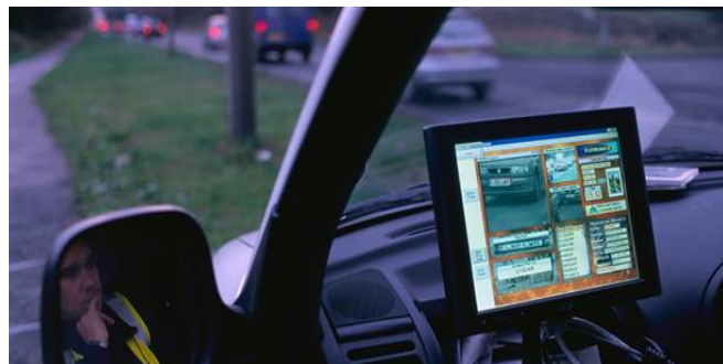
Figure 8 - An ALPR system monitors the roads of Manchester, England, checking motorists identity compared to three databases. Photo courtesy of MSNBC. http://www.msnbc.msn.com/id/1522111/
