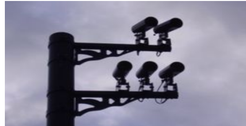
Figure 4 - Congestion Charge CCTV cameras near Vauxhall Bridge. Photo provided by Transport for London.
