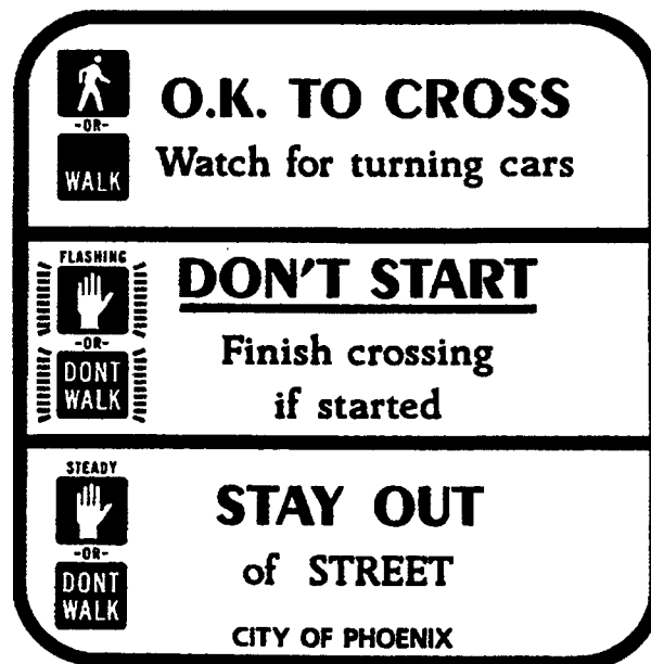
Figure 3. Phoenix pedestrian signal explanation sign.
