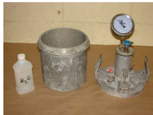
Figure 2 Pressure meter (ASTM C 231)
