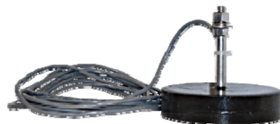
A uniquely coded transmitter is attached to the underside of the transit vehicle.
