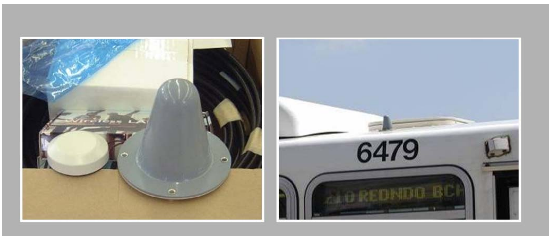
Figure 4-10: Typical GPS and Wireless Communications Antenna Installation
