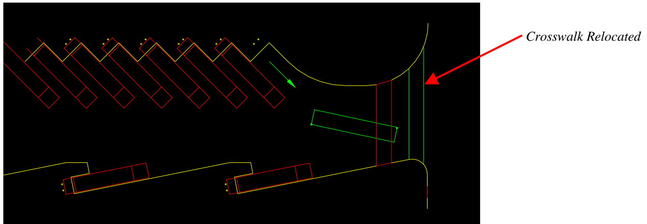
Figure 10, Entrance Crosswalk Relocated
