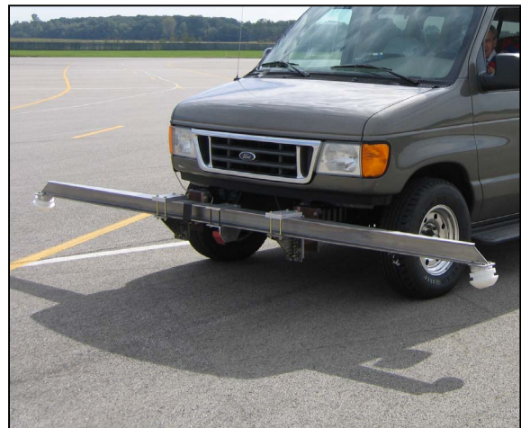
Figure 3.3. “Heavy-Duty” outrigger installed on the front of a 2003 Ford E-350.
